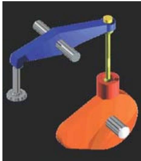
A rocker using a cam.
