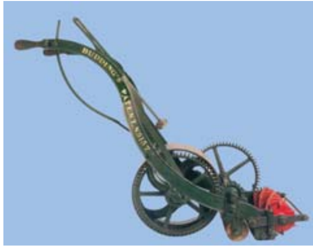
Lawn-mover is a combination of kinematic links.
