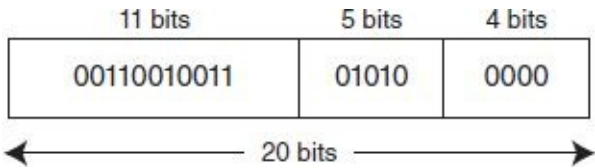
FIGURE 6.14 The Address 0x326A0 from Example 6.6 Divided into Fields for Direct Mapping
