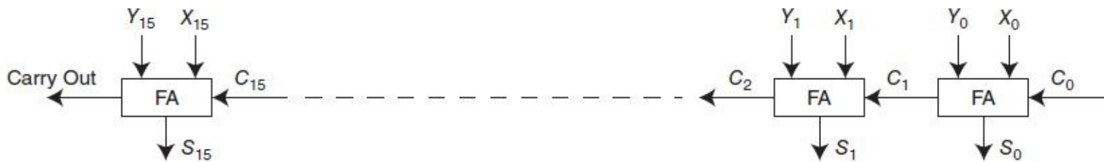
FIGURE 3.13 Logic Diagram for a Ripple-Carry Adder
