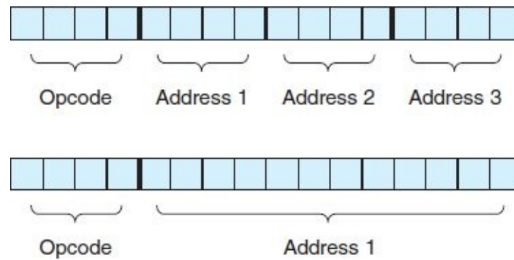
FIGURE 5.2 Two Possibilities for a 16-Bit Instruction Format
