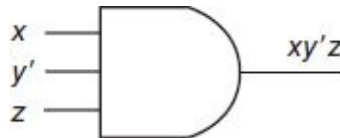
FIGURE 3.7 A Three-Input AND Gate Representing x y' z
