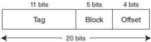
FIGURE 6.13 Direct Mapped Memory Format for Example 6.6
