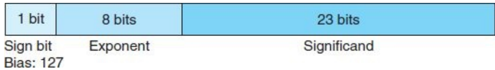
FIGURE 2.2 IEEE-754 Single-Precision Floating-Point Representation
