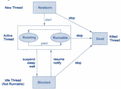
Fig. 12.3 State transition diagram of a thread
