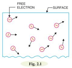
However, if sufficient external energy is given to the free electron, its kinetic energy is increased and thus electron will cross over the surface barrier to leave the metal. This additional energy required by an electron to overcome the surface barrier of the metal is called *work function* of the metal.
