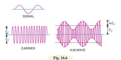
The amplitude of the carrier wave varies at signal frequency  $f_s$ . Therefore, the amplitude of AM wave is given by :
