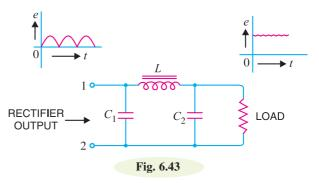
(a) The *filter capacitor*  $C_1$  offers low reactance to a.c. component of rectifier output while it offers infinite reactance to the d.c. component. Therefore, capacitor  $C_1$  bypasses an appreciable amount of a.c. component while the d.c. component continues its journey to the choke L.
