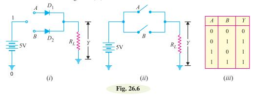
(*ii*) When A is connected to ground and B connected to the positive terminal of the battery, diode  $D_2$  is forward biased and diode  $D_1$  is non-conducting. Therefore, diode  $D_2$  conducts and the output voltage is ideally +5 V. In terms of binary, when A = 0 and B = 1, then Y = 1 [See Fig. 26.6 (*iii*)].
