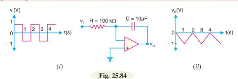
Solution. The output voltage of this circuit is given by;
