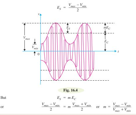
**Example 16.2.** The maximum peak-to-peak voltage of an AM wave is 16 mV and the minimum peak-to-peak voltage is 4 mV. Calculate the modulation factor.
