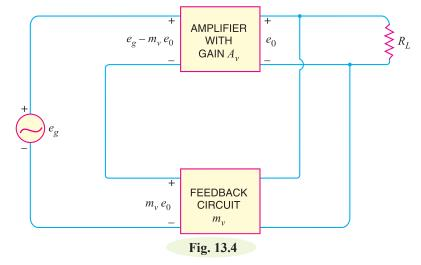
But  $e_0/e_{\sigma}$  is the voltage gain of the amplifier with feedback.
