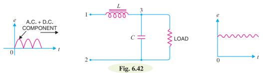
At terminal 3, the rectifier output contains d.c. component and the remaining part of a.c. component which has managed to pass through the choke. Now, the low reactance of filter capacitor bypasses the a.c. component but prevents the d.c. component to flow through it. Therefore, only d.c. component reaches the load. In this way, the filter circuit has filtered out the a.c. component from the rectifier output, allowing d.c. component to reach the load.
