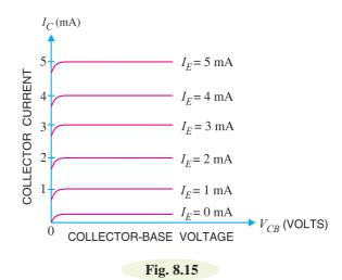
(*iii*) A very large change in collector-base voltage produces only a tiny change in collector current. This means that output resistance is very high.
