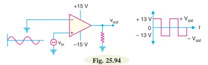
When the input signal goes positive, the output jumps to about + 13 V. When the input goes negative, the output jumps to about - 13 V. The output changes rapidly from - 13 V to + 13 V and *vice-versa*. This change is so rapid that we get a square wave output for a sine wave input.
