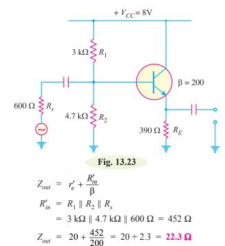
$Z_{out} = 20 + \frac{432}{200} = 20 + 2.3 = 22.3 \Omega$ Note that output impedance of the emitter follower is very low. On the other hand, it has high input impedance. This property makes the emitter follower a perfect circuit for connecting a low impedance load to a high-impedance source.
