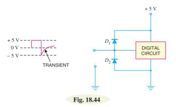
Fig. 18.44 shows the protection of a typical digital circuit against transients by the diode clipper. When the transient shown in Fig. 18.44 occurs on the input line, it causes diode  $D_2$  to be forward biased. The diode  $D_2$  will conduct; thus shorting the transient to the ground. Consequently, the input of the circuit is protected from the transient.
