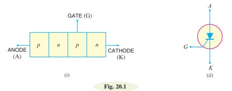
change alternating current into direct current and at the same time can control the amount of power fed to the load. Thus *SCR* combines the features of a rectifier and a transistor.
