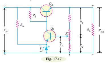
Operation. The unregulated d.c. supply is fed to the voltage regulator. The circuit maintains constant output voltage irrespective of the variations in load or input voltage. Here is how the circuit operates.
