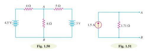
Fig. 1.51 shows Norton's equivalent circuit of a network behind terminals A and B. Convert it into Thevenin's equivalent circuit.
