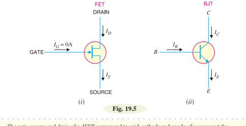
The gate, source and drain of a *JFET* correspond to grid, cathode and anode of a vacuum tube.
