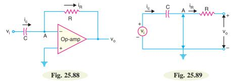
Circuit analysis. Since point A in Fig. 25.88 is at virtual ground, the virtual-ground equivalent circuit of the operational differentiator will be as shown in Fig. 25.89. Because of virtual ground and infinite impedance of OP-amp, all the input current  $i_c$  flows through the feedback resistor R i.e.  $i_c = i_R$ .
