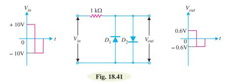
Thus for the input voltage waveform, the output voltage varies between -0.6V and 0.6V. This circuit is sometimes used to convert a sine-wave input to a reasonably square-wave output signal.
