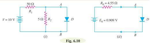
Solution. We shall use Thevenin's theorem to find current in the diode. Referring to Fig. 6.10(*i*),
