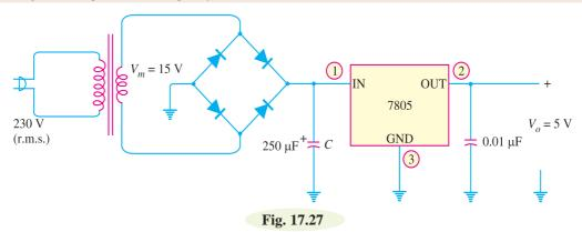
**Solution.** The resulting circuit is shown in Fig. 17.27. Here we use 7805 *IC* with unregulated power supply.
