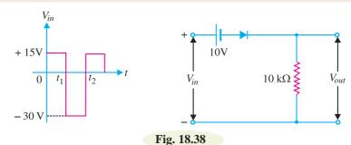
**Solution.** For any value of  $V_{in} > 10V$ , the ideal diode is forward biased and  $V_{out} = V_{in} - 10$ . For any value of  $V_{in} < 10V$ , the ideal diode is reverse biased and  $V_{out} = 0$ .
