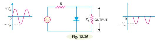
The circuit action is as follows. During the positive half-cycle of the input voltage, the diode is forward biased and conducts heavily. Therefore, the voltage across the diode (which behaves as a short) and hence across the load  $R_I$  is zero. Hence \*output voltage during positive half-cycles is zero.
