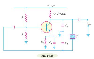
resonance caused by L and  $(C_1 + C_2)$ , we have the parallel resonance of the crystal. At parallel resonance, the impedance of the crystal is maximum. This means that there is a maximum voltage drop across  $C_1$ . This in turn will allow the maximum energy transfer through the feedback network at  $f_p$ .
