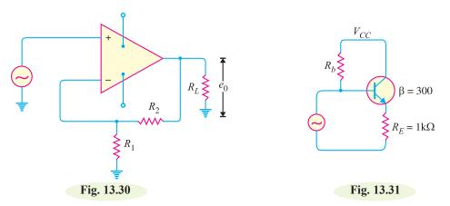
6. Fig. 13.30 shows the negative feedback amplifier. If the gain of the amplifier without feedback is  $10^5$  and  $R_1 = 100 \Omega$ ,  $R_2 = 100 k\Omega$ , find (*i*) feedback fraction (*ii*) gain with feedback.
