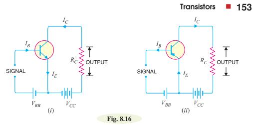
1. Base current amplification factor ( $\beta$ ). In common emitter connection, input current is  $I_B$  and output current is  $I_C$ .
