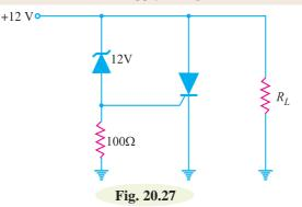
**Solution.** The breakdown voltage of the zener diode is 12V and it has a tolerance of  $\pm$  10%. It means that breakdown voltage of zener can vary from 10.8V to 13.2V. Since the trigger voltage of *SCR* has a maximum value of 1.5 V,
