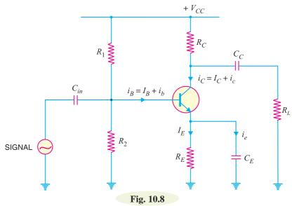
(*i*) **D. C. equivalent circuit.** In the d.c. equivalent circuit of a transistor amplifier, only d.c. conditions are to be considered *i.e.* it is presumed that no signal is applied. As direct current cannot flow through a capacitor, therefore, *all the capacitors look like open circuits in the d.c. equivalent circuit.* It follows, therefore, that in order to draw the equivalent d.c. circuit, the following two steps are applied to the transistor circuit :
