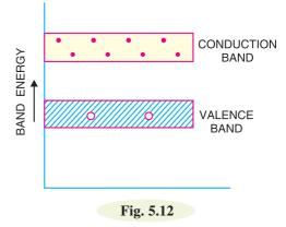
(*ii*) Thermal energy of room temperature still generates a few hole-electron pairs. However, the number of free electrons provided by the pentavalent impurity far exceeds the number of holes. It is due to this predominance of electrons over holes that it is called *n*-type semiconductor (*n* stands for negative).
