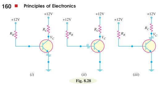
**Solution.** Fig. 8.28 shows the short circuit failures in a transistor. We shall discuss the circuit behaviour in each case.
