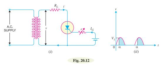
**Operation.** The a.c. supply to be converted into d.c. supply is applied to the primary of the transformer. Suppose the peak reverse voltage appearing across secondary is less than the reverse
