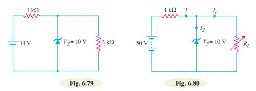
**15.** In the circuit shown in Fig. 6.80, determine the range of  $R_L$  that will result in a constant voltage of 10 V across  $R_L$ . **[250 \Omega to 1.25 k\Omega]**
