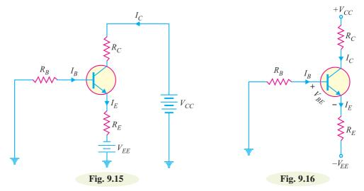
We shall first redraw the circuit in Fig. 9.15 as it usually appears on schematic diagrams. This means deleting the battery symbols as shown in Fig. 9.16. All the information is still (See Fig. 9.16) on the diagram except that it is in condensed form. That is a negative supply voltage  $-V_{EE}$  is applied to the bottom of  $R_E$  and a positive voltage of  $+V_{CC}$  to the top of  $R_C$ .
