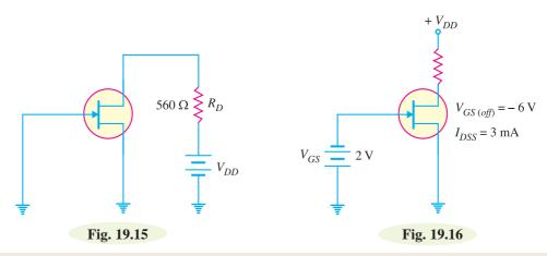
Example 19.5. Determine the value of drain current for the circuit shown in Fig. 19.16. **Solution.** It is clear from Fig. 19.16 that  $V_{GS} = -2V$ . The drain current for the circuit is given by;
