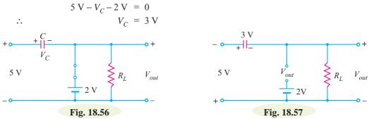
Therefore, the capacitor will charge up to 3 V.
