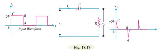
Let us look at the physical explanation of this behaviour of the circuit. Since time constant RC of the circuit is very small w.r.t. time period of input wave and  $X_C >> R$ , the capacitor will become fully charged during the early part of each half-cycle of the input wave. During the remainder part of the
