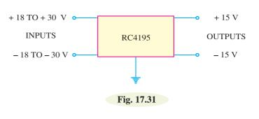
are  $\pm$  15V. The data sheet of an *RC* 4195 lists a maximum output current of 150 mA for each supply and a load regulation of 3mV. Adjustable dual-tracking regulators are also available. These regulators have outputs that can be varied between their two rated limits.
