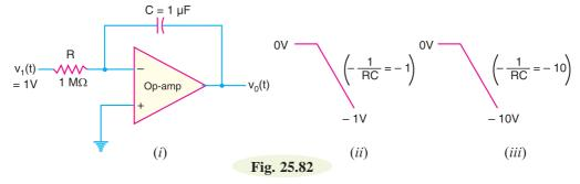
If the scale factor is changed by making  $R = 100 \text{ k}\Omega$ , then,
