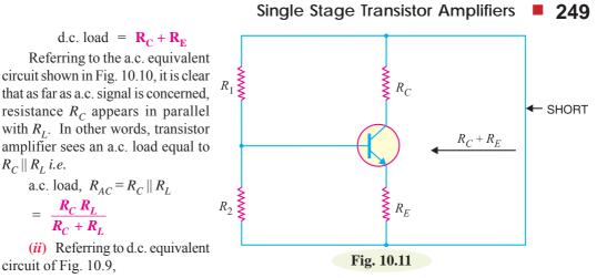
$$V_{CC} = V_{CE} + I_C \left( R_C + R_E \right)$$
