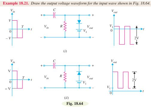
**Solution.** Fig. 18.64 (*i*) shows the output voltage waveform for the input wave to the clamping circuit. This is a negative clamper and pushes the input wave downward so that positive peak voltage is now  $V_1$ . Fig. 18.64 (*ii*) shows the output voltage waveform from a positive clamper. Note that the input wave is pushed upwards so that negative peaks are  $V_1$  volts above the zero level.
