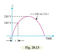
**Example 20.8.** In an SCR half-wave rectifier circuit, what peak-load current will occur if we measure an average (d.c.) load current of 1A at a firing angle of  $30^{\circ}$ ?
