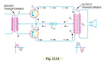
It may be noted here that push-pull arrangement also permits a maximum transfer of power to the load through impedance matching. If  $R_L$  is the resistance appearing across secondary of output transformer, then resistance  $R'_L$  of primary shall become :
