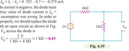
We know that 0.7V is required to turn ON the diode. Since  $V_D$  is only 0.4V, the answer confirms that the diode is OFF.
