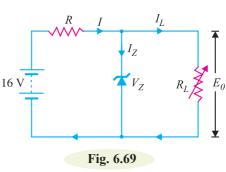
The voltage across *R* is to remain constant at 16 - 12 = 4 V as the load current changes from 0 to 200 mA. The minimum zener current will occur when the load current is maximum.
