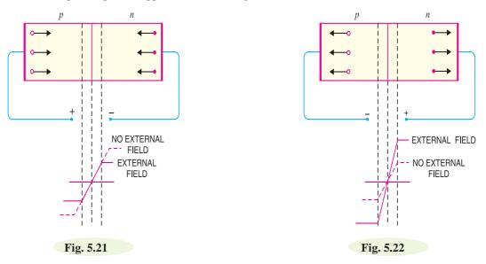
**2. Reverse biasing.** When the external d.c. voltage applied to the junction is in such a direction that potential barrier is increased, it is called **reverse biasing.**
