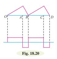
of the input wave, its amplitude changes at a constant rate and, therefore, the differentiated wave has a constant value for each constant rate of change. During the period *AB* of the input wave, the change is less abrupt so that the output will be a very narrow pulse of rectangular form. Thus when a triangular wave is fed to a differentiating circuit, the output consists of a succession of rectangular waves of equal or unequal duration depending upon the shape of the input wave.
