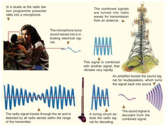
receivers are called A.M. radio receivers. In order to reproduce the A.M. wave into sound waves, every radio receiver must perform the following functions :
