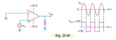
From the input/output waveforms, you can see that every time the input crosses 0 V going positive, the output jumps to + 13 V. Similarly, every time the input crosses 0 V going negative, the output jumps to -13 V. Since the change (+ 13 V or -13 V) occurs every time the input crosses 0 V, we can tell when the input signal has crossed 0 V. Hence the name zero-crossing detector.
