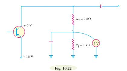
The circuit is not operating properly. It is because the voltage at point B should be 2 V instead of 4V.
