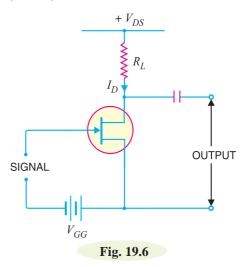
$V_{GG}$  in the gate circuit or by a circuit known as biasing circuit. In the present case, we are providing biasing by the battery  $V_{GG}$ .
