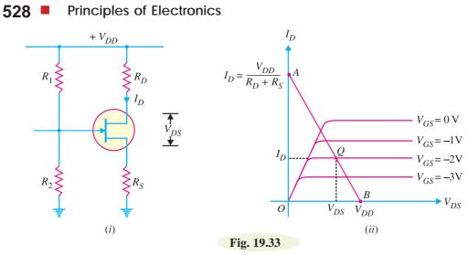
As for a given circuit,  $V_{DD}$  and  $(R_D + R_s)$  are constant, therefore, exp. (i) is a first degree equation and can be represented by a straight line on the drain characteristics. This is known as d.c. load line for JFET and determines the locus of  $I_D$  and  $V_{DS}$  (*i.e.* operating point) in the absence of the signal. The d.c. load line can be readily plotted by locating the two end points of the straight line.
