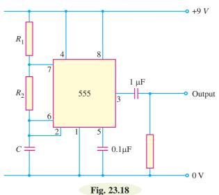
The time  $T_1$  for which the output is 'high' is given by ;  $T_1 = 0.694 (R_1 + R_2) C$ The time  $T_2$  for which the output is 'low' is given by ;
