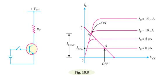
(i) **OFF region.** When the input base voltage is zero or \*negative, the transistor is said to be in the OFF condition. In this condition,  $I_B = 0$  and the collector current is equal to the collector leakage current  $I_{CEO}$ . The value of  $I_{CEO}$  can be obtained from the characteristics if we know  $V_{CF}$ .
