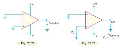
There are several methods that may be used to eliminate output offset voltage. One of these is to apply an *input offset voltage* between the input terminals of DA (or OP- amp) so as to make output 0V as shown in Fig. 25.23. The value of input offset voltage  $(V_{i0})$  required to eliminate the output offset voltage is given by;
