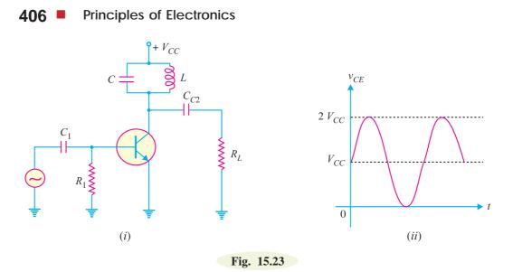
As discussed earlier,  $P_D$  in class C operation is very small because the transistor remains biased off during most of the input signal cycle. Consequently,  $P_D$  may be neglected as compared to  $P_{o(max)}$ .
