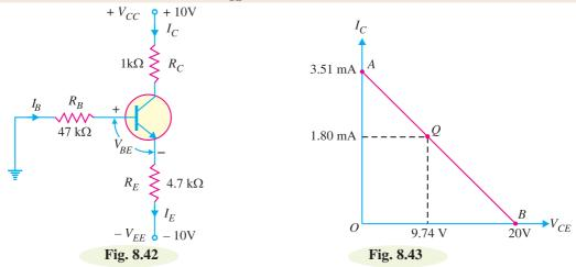
The presence of two power supplies has an effect on the baisc equations for  $I_C$  and  $V_{CE}$  used for single power supply (*i.e.*  $V_{CC}$ ). Normally, the two supply voltages will be equal. For example, if  $V_{CC} = +10V$  (d.c.), then  $V_{EE} = -10$  V (d.c.).
