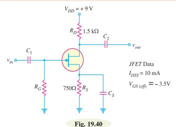
**Solution.** From the d.c. bias analysis, we get,  $*I_D = 2.3$  mA and  $V_{GS} = -1.8$ V. The value of  $g_m$  is given by;
