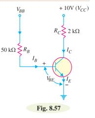
Collector voltage,  $V_C = V_{CC} - I_C R_C$
