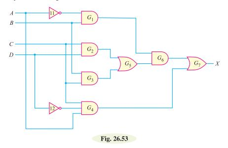
**Step 1.** Apply distributive law to the second term by multiplying the term CD + BC by  $\overline{AB}$ . The result is :
