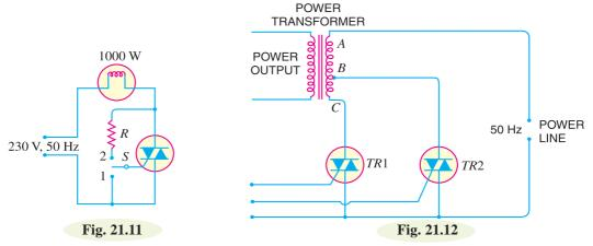
(*i*) As a high-power lamp switch. Fig. 21.11 shows the use of a triac as an a.c. on/off switch. When switch S is thrown to position 1, the triac is cut off and the output power of lamp is zero. But as the switch is thrown to position 2, a small gate current (a few mA) flowing through the gate turns the triac on. Consequently, the lamp is switched on to give full output of 1000 watts.
