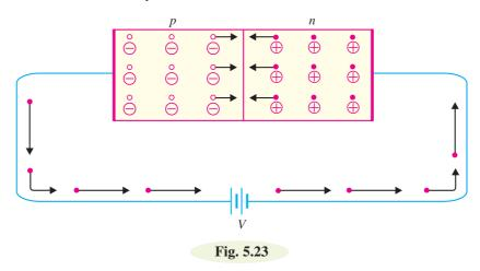
The mechanism of current flow in a forward biased pn junction can be summed up as under :
