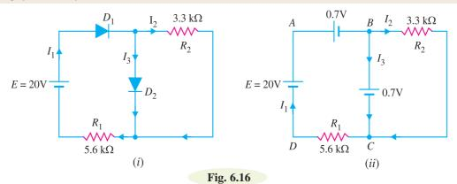
**Solution.** An inspection of the circuit shown in Fig. 6.16 (*i*) shows that both diodes  $D_1$  and  $D_2$  are forward biased. Using simplified model for the diodes, the circuit shown in Fig. 6.16 (*i*) becomes the one shown in Fig. 6.16 (*ii*). The voltage across  $R_2$  (= 3.3 k  $\Omega$ ) is 0.7V.
