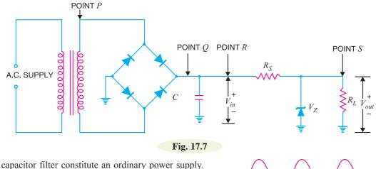
However, when voltage regulating device is added to this ordinary power supply, it turns into a regulated power supply.
