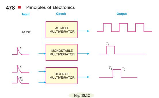
*(iii)* The bistable multivibrator has both the two states stable. It requires the application of an external triggering pulse to change the operation from either one state to the other. Thus one pulse is used to generate half-cycle of square wave and another pulse to generate the next half-cycle of square wave. It is also known as a *flip-flop multivibrator* because of the two possible states it can assume.
