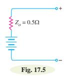
**Example 17.6.** A d.c. power supply is delivering 10V (normally) to a load that is varying sinusoidally between 0.5A and 1 A at a rate of 10 kHz. If the output impedance of the power supply is  $0.01\Omega$  at 10 kHz, determine the fluctuations in the output voltage caused by this periodic load change.
