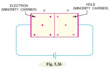
characteristic. This is called *reverse* \*saturation current  $(I_s)$  and is due to the minority carriers. It may be recalled that there are a few free electrons in *p*-type material and a few holes in *n*-type material. These undesirable free electrons in *p*-type and holes in *n*-type are called *minority carriers*. As shown in Fig. 5.26, to these minority carriers, the applied reverse bias appears as forward bias. Therefore, a \*\*small current flows in the reverse direction.
