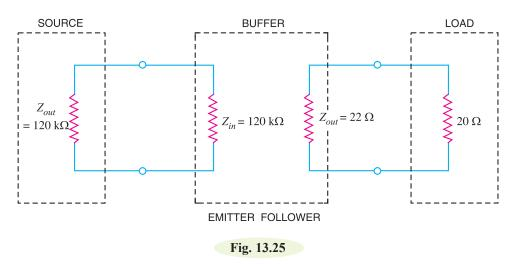
It may be noted that the job of impedance matching can also be accomplished by a transformer. However, emitter follower is preferred for this purpose. It is because emitter follower is not only more convenient than a transformer but it also has much better frequency response *i.e.*, it works well over a large frequency range.
