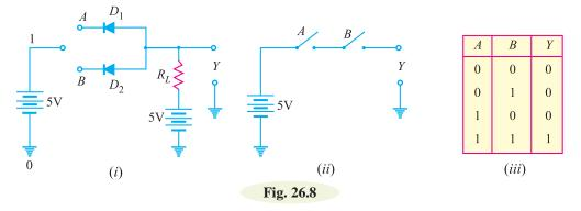
(*i*) When both A and B are connected to ground, both the diodes  $(D_1 \text{ and } D_2)$  are forward biased and hence they conduct current. Consequently, the two diodes are grounded and output voltage is zero. In terms of binary, when A = 0 and B = 0, then Y = 0 as shown in truth table in Fig. 26.8 (*iii*).
