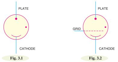
Fig. 3.1 shows the schematic symbol for a cold-cathode gas diode, known as *glow tube*. The dot within the circle indicates the presence of gas. Fig. 3.2 shows the schematic symbol of cold-cathode gas triode, known as *grid glow tube*.
