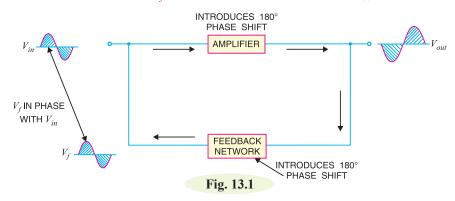
The positive feedback increases the gain of the amplifier. However, it has the disadvantages of increased distortion and instability. Therefore, positive feedback is seldom employed in amplifiers. One important use of positive feedback is in oscillators. As we shall see in the next chapter, if positive feedback is sufficiently large, it leads to oscillations. As a matter of fact, an oscillator is a device that converts d.c. power into a.c. power of any desired frequency.
