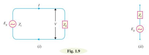
The opposition to load current inside the a.c. source is called its *internal impedance*  $Z_i$ . The equivalent circuit of an a.c. source is the generated *e.m.f.*  $E_g(r.m.s.)$  in series with internal impedance  $Z_i$  of the source as shown in Fig. 1.9 (*ii*). Referring to Fig. 1.9 (*i*), it is clear that :
