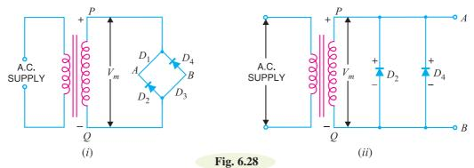
Referring to Fig. 6.28 (*ii*), it is clear that two reverse biased diodes (*i.e.*,  $D_2$  and  $D_4$ ) and the secondary of transformer are in parallel. Hence PIV of each diode ( $D_2$  and  $D_4$ ) is equal to the maximum voltage ( $V_m$ ) across the secondary. Similarly, during the next half cycle,  $D_2$  and  $D_4$  are forward biased while  $D_1$  and  $D_3$  will be reverse biased. It is easy to see that reverse voltage across  $D_1$  and  $D_3$  is equal to  $V_m$ .
