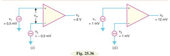
Solution. Fig. 25.36(i) shows the differential-mode operation whereas Fig. 25.36(ii) shows the
