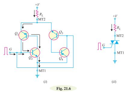
Fig. 21.6 (*ii*) shows the action of triac (*MT*2 positive w.r.t. *MT*1) by replacing the triac with its symbol.
