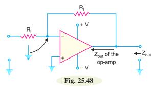
parallel combination of  $R_f$  and the output impedance of OP-amp itself.
