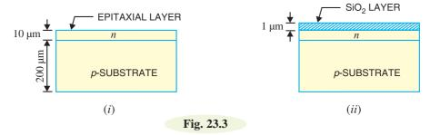
semi-conductor on the heated surface of substrate [See Fig. 23.3 (*i*)]. This thin layer is called the *\*epitaxial layer* and is about 10  $\mu$ m thick. It is in this layer that the whole integrated circuit is formed.
