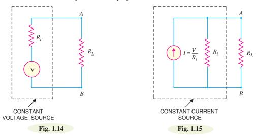
(*ii*) If in Fig. 1.14, the load is short-circuited (*i.e.*  $R_L = 0$ ), the short circuit current is given by:
