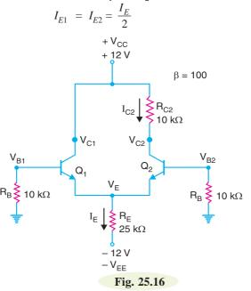
Ignoring the base current, the emitter voltage for both transistors is  $V_E = -0.7$  V.
