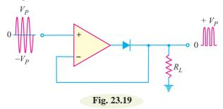
When the input signal goes positive, the output of Op-Amp goes positive and turns on the diode. The circuit then acts like a voltage follower and the positive half-cycle appears across the load resistor  $R_L$ . On the other hand, when the input goes negative, the Op-Amp output goes negative and turns off the diode. Since the diode is open, no voltage appears across the load resistor  $R_L$ . Therefore, the voltage across  $R_L$  is almost a perfect half-wave signal.
