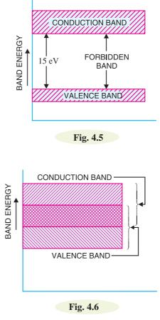
comparatively smaller electric field (smaller than insulators but much greater than conductors) is required to push the electrons from the valence band to the conduction band. In short, a semiconductor has :
