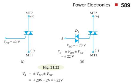
Therefore, in order to turn on the triac, the gate trigger signal  $V_A$  must be  $\pm$  22V. Note that triac triggering control is the primary function of a diac.
