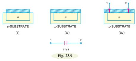
(*iv*) **Capacitors.** Fig. 23.9 shows the process of fabricating a capacitor in the monolithic *IC*. The first step is to diffuse an *n*-type material into the substrate which forms one plate of the capacitor as shown in Fig. 23.9 (*i*). Then  $SiO_2$  layer is re-formed over the wafer by passing pure oxygen as shown in Fig. 23.9 (*ii*).
