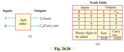
The half adder would behave according to the truth table shown in Fig. 26.56 (*ii*). Take a careful look at the truth table. The output columns (sum and carry) can be produced by using two gates as under :
