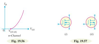
**Schematic Symbols.** Fig. 19.57 (*i*) shows the schematic symbols for *n*-channel *E-MOSFET* whereas Fig. 19.57 (*ii*) shows the schematic symbol for *p*-channel *E-MOSFET*. When  $V_{GS} = 0$ , the *E-MOSFET* is *OFF* because there is no conducting channel between source and drain. The broken channel line in the symbols indicates the normally *OFF* condition.
