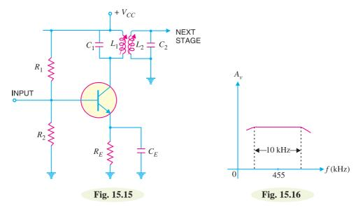
When two resonant circuits are critically coupled, the frequency response becomes flat over a considerable range of frequencies as shown in Fig. 15.16. In other words, the double tuned circuit has better frequency response as compared to that of a single tuned circuit. The use of double tuned circuit offers the following advantages :
