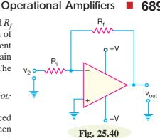
**OP-Amp Input/Output Polarity Relationship**. The polarity relationship between  $v_1$  and  $v_2$ 2. will determine whether the OP-amp output voltage polarity is positive or negative. There is an easy method for it. We know the differential input voltage  $v_{in}$  is the difference between the non-inverting input  $(v_1)$  and inverting input  $(v_2)$  *i.e.*,
