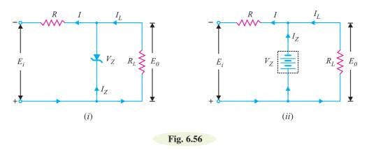
When the circuit is properly designed, the load voltage  $E_0$  remains essentially constant (equal to  $V_Z$ ) even though the input voltage  $E_i$  and load resistance  $R_L$  may vary over a wide range.
