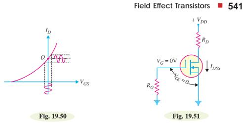
We can use the simple circuit of Fig. 19.51 to provide zero bias. This circuit has  $V_{GS} = 0$  V and  $I_D = I_{DSS}$ . We can find  $V_{DS}$  as under :
