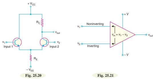
The differential amplifier amplifies the difference between the two input voltages. This point is illustrated in Fig. 25.21. The difference between the input voltages is  $v_{in} = v_1 - v_2 i.e.$ ,
