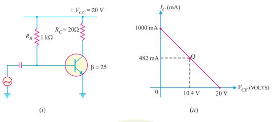
**Solution.** First draw the *d.c.* load line by locating the two end points *viz.*,  $I_{C (sat)} = V_{CC}/R_{C} =$  $20 \text{ V}/20 \Omega = 1 \text{ A} = 1000 \text{ mA} \text{ and } V_{CE} = V_{CC} = 20 \text{ V}$  as shown in Fig. 12.7 (*ii*). The operating point Q of the circuit can be located as under :
