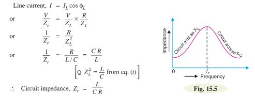
Thus at parallel resonance, the circuit impedance is equal to L/CR. It may be noted that  $Z_r$  will be in ohms if R, L and C are measured in ohms, henry and farad respectively.
