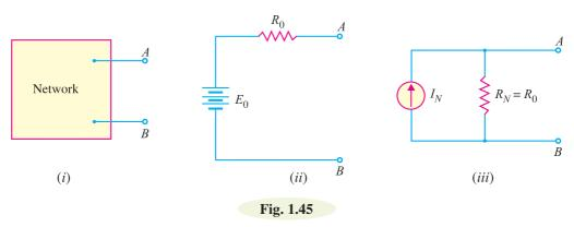
(ii) To convert Norton's equivalent circuit into Thevenin's equivalent circuit,
