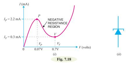
(*iii*) When forward bias is increased beyond valley-point voltage  $V_V$  (= 0.7 V), the tunnel diode behaves as a normal diode. In other words, from point V onwards, the diode current increases with the increase in forward voltage *i.e.*, the diode exhibits positive resistance once again. Fig. 7.18. (*ii*) shows the symbol of tunnel diode. It may be noted that a tunnel diode has a high reverse current but operation under this condition is not generally used.
