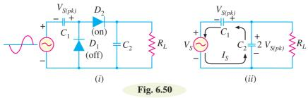
Referring to Fig. 6.50 (*ii*), it is easy to see that  $C_1$  (charged to  $V_{S(pk)}$ ) and the source voltage ( $V_S$ ) now act as *series-aiding* voltage sources. Thus  $C_2$  will be charged to the sum of the series peak voltages *i.e.* 2  $V_{S(pk)}$ .
