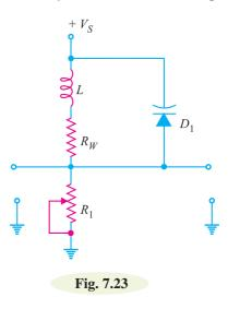
circuit is the *winding resistance* of the inductor. This winding resistance is in series with the potentiometer  $R_1$ . Thus  $R_1$  and  $R_W$  form a voltage divider that is used to determine the amount of reverse bias across the varactor diode  $D_1$  and therefore its capacitance. By adjusting the setting of  $R_1$ , we can vary the diode capacitance. This, in turn, varies the resonant frequency of the *LC* circuit. The resonant frequency  $f_r$  of the *LC* circuit is given by;
