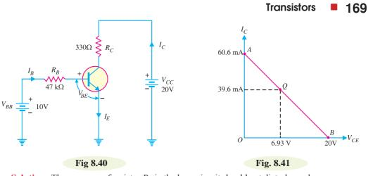
**Solution.** The presence of resistor  $R_{R}$  in the base circuit should not disturb you because we can apply Kirchhoff's voltage law to find the value of  $I_B$  and hence  $I_C (= \beta I_B)$ . Referring to Fig. 8.40 and applying Kirchhoff's voltage law to base-emitter loop, we have,
