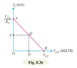
\* Why load line? The resistance  $R_c$  connected to the device is called load or load resistance for the circuit and, therefore, the line we have just constructed is called the load line.
