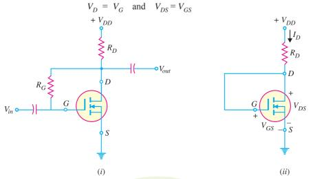
The value of drain-source voltage  $V_{DS}$  for the drain-feedback circuit is
