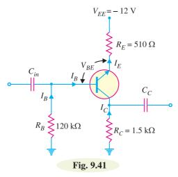
Solution. Such a problem should not pose any difficulty. We are to simply find the d.c. values. Note that capacitors behave as open to d.c. Applying Kirchhoff's voltage law to the path passing through  $R_B$ ,  $V_{BE}$ ,  $R_E$  and  $V_{EE}$ , we have,
