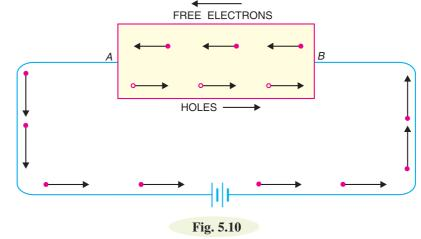
and combine with holes, thus cancelling them. At the same time, the loosely held electrons near the positive terminal *A* are attracted away from their atoms into the positive terminal. This creates new holes near the positive terminal which again drift towards the negative terminal.
