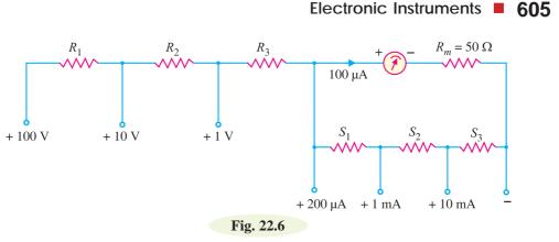
Here the full-scale deflection (*f.s.d.*) current of the meter is  $100 \,\mu\text{A}$  and meter resistance is  $50 \,\Omega$ . The design of this multimeter means finding the values of various resistances.
