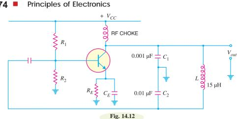
Example 14.4. A 1 mH inductor is available. Choose the capacitor values in a Colpitts oscillator so that f = 1 MHz and  $m_v = 0.25$ .
