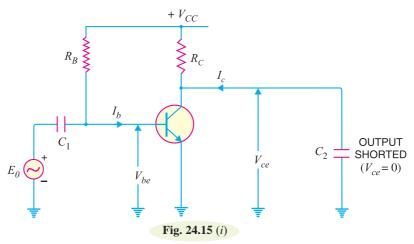
Substituting  $V_{ce} = 0$  in equations (i) and (ii) above, we get,
