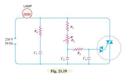
The circuit action is as follows : As the input voltage increases positively or negatively,  $C_1$  and  $C_2$  charge at a rate determined primarily by  $R_2$ . When the voltage across  $C_3$  exceeds the breakover voltage of the diac, the diac is fired into the conducting state. The capacitor  $C_3$  discharges through the conducting diac into the gate of the triac. Hence, the triac is turned on to pass the a.c. power to the
