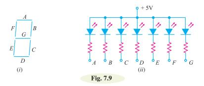
Fig. 7.9 (*ii*) shows the schematic diagram of seven-segment display. External series resistors are included to limit currents to safe levels. Note that the anodes of all seven LEDs are connected to a
