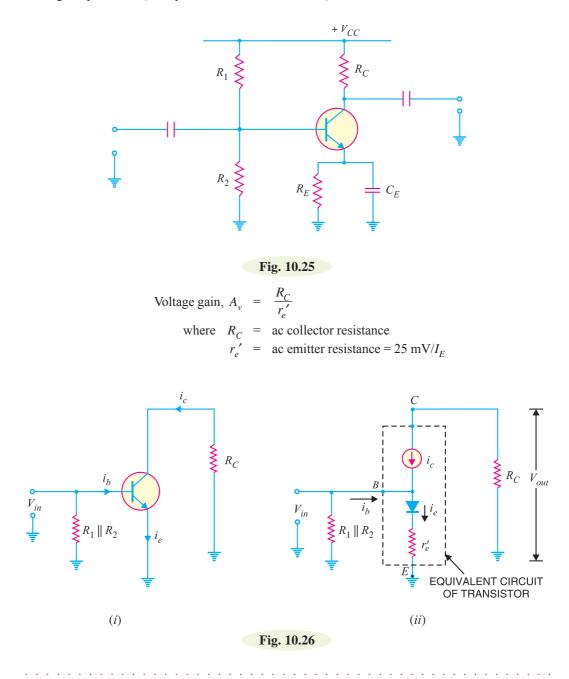
\* The size of  $C_E$  is so selected that it offers negligible reactance to the frequencies handled by the amplifier (See Example 10.2).
