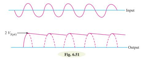
The voltage multipliers have the disadvantage of poor voltage regulation. This means that d.c. output voltage drops considerably as the load current increases. Large filter capacitors are needed to help maintain the output voltage.
