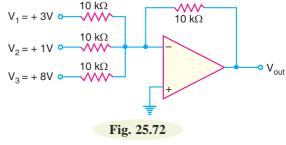
$$V_{out} = -(V_1 + V_2 + V_3) = -(3 + 1 + 8) = -12 V$$
