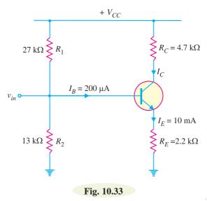
**Solution.** In most practical circuits, the value of a.c. emitter resistance  $r'_e$  for the transistor is generally quite small as compared to  $R_E$  and can be neglected in circuit calculations with reasonable accuracy.
