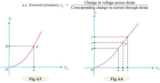
The a.c. forward resistance is more significant as the diodes are generally used with alternating voltages. The a.c. forward resistance can be determined from the forward characteristic as shown in Fig. 6.6. If *P* is the operating point at any instant, then forward voltage is *ob* and forward current is *oe*. To find the a.c. forward resistance, vary the forward voltage on both sides of the operating point equally as shown in Fig. 6.6 where ab = bc. It is clear from this figure that :
