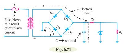
**Solution.** The common faults in a zener voltage regulator are shorted filter capacitor or opened filter capacitor.
