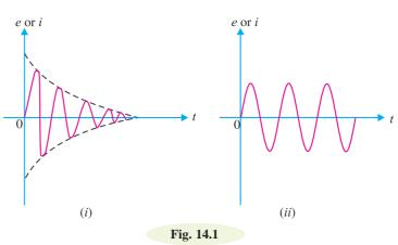
lation. Further, no means are provided to compensate for the losses and consequently the amplitude of the generated wave decreases gradually. It may be noted that frequency of oscillations remains unchanged since it depends upon the constants of the electrical system.
