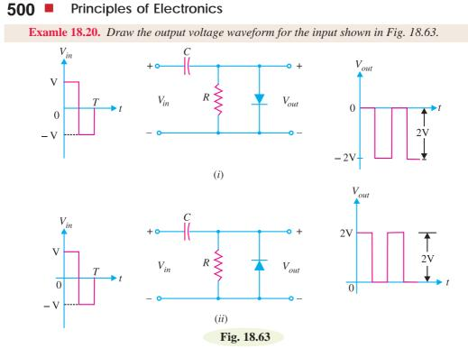
**Solution.** Fig. 18.63 (*i*) shows the output voltage waveform for the input wave to the clamping circuit. Note that it is a negative clamper and pushes the input wave downwards so that positive peaks fall on the zero level. Fig. 18.63 (*ii*) shows the output voltage waveform for the input wave to a positive clamper. The clamper pushes the input wave upwards so that the negative peaks fall on the zero level.
