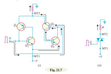
Fig. 21.7 (*ii*) shows the action of triac (*MT*2 negative w.r.t. *MT*1) by replacing the triac with its symbol.
