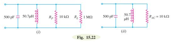
The equivalent circuit is shown in Fig. 15.22 (i). This further reduces to the circuit shown in Fig. 15.22 (ii).
