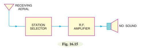
From the above discussion, it follows that audio signal must be separated from the carrier at a suitable stage in the receiver. The recovered audio signal is then amplified and fed to the speaker for conversion into sound.
