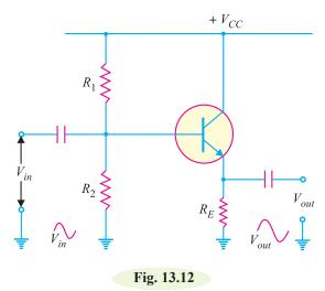
(*i*) There is neither collector resistor in the circuit nor there is emitter bypass capacitor. These are the two circuit recognition features of the emitter follower.
