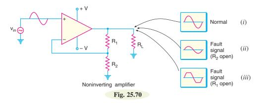
(*ii*) When  $R_2$  is open: If  $R_2$  opens, the feedback circuit would consist solely of  $R_1$ . In this case, the gain would *drop*. It is because the circuit would now act as a \*voltage follower. In other words, the circuit would now be a buffer with an output voltage that is equal to the input voltage. Thus we would have the output signal as shown in Fig. 25.70 (*ii*). The waveform would be correct but we would have unity gain.
