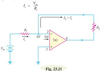
The internal impedance of Op-Amp is extremely high (ideally infinite) so that practically all of  $I_i$  flows through  $R_L$ . Since  $I_i = I_L$ ,
