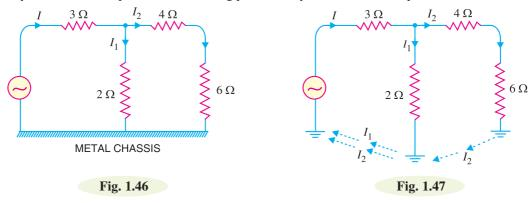
It is customary to refer to the chassis as *ground*. Fig. 1.47 shows the symbol for chassis. It may be seen that all points connected to chassis are shown as grounded and represent the same potential. The adoption of this scheme (*i.e.* showing points of same potential as grounded) often simplifies the electronic circuits. In our further discussion, we shall frequently use this scheme.
