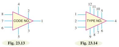
Fig. 23.13 shows the symbol of an *IC r-f* amplifier containing 3 transistors, 3 resistors and 8 terminals. Similarly, Fig. 23.14 shows an *IC* audio amplifier which contain 6 transistors, 2 diodes, 17 resistors and has 12 terminals.
