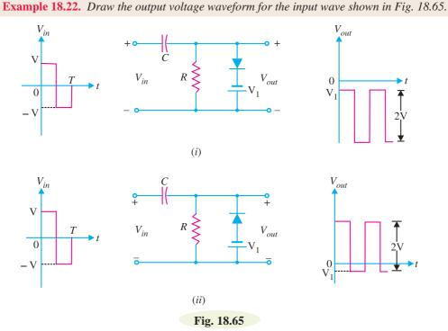
**Solution.** Fig. 18.65 (*i*) shows the output voltage waveform for the input wave to the clamping circuit. This is a negative clamper and pushes the input wave downward so that positive peaks lie  $V_1$  volts below the zero level. Fig. 18.65 (*ii*) shows the output voltage waveform from a positive clamper. Note that the input waveform is pushed upwards so that negative peaks lie  $V_1$  volts below zero level.
