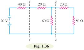
We can again replace the circuit to the left of *YY* in Fig. 1.35 by its Thevenin's equivalent circuit. Therefore, the original circuit reduces to that shown in Fig. 1.36.
