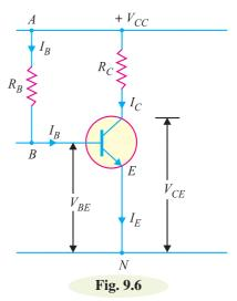
It may be noted that  $V_{CC}$  is a fixed known quantity and  $I_B$  is chosen at some suitable value. Hence,  $R_B$  can always be found directly, and for this reason, this method is sometimes called *fixed-bias method*.
