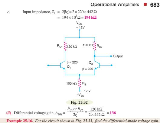
**Solution.** Because we are taking the output from  $Q_2$ , there is no need for collector resistor on  $Q_1$ . To find the relevant bias currents, we set the input sources to 0V, connecting the two bases to ground.
