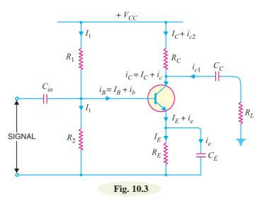
(iii) Emitter bypass capacitor  $C_E$ . An emitter bypass capacitor  $C_E (\simeq 100 \mu F)$  is used in parallel with  $R_E$  to provide a low reactance path to the amplified a.c. signal. If it is not used, then amplified a.c. signal flowing through  $R_E$  will cause a voltage drop across it, thereby reducing the output voltage.
