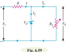
(i)  $\mathbf{R}_{Lmin}$  and  $\mathbf{I}_{Lmax}$ . Once the zener is in the "on" state, load voltage  $E_0 (= V_Z)$  is constant. As a result, when load resistance is minimum (*i.e.*,  $R_{Lmin}$ ), load current will be maximum ( $I_L = E_0/R_L$ ). In order to find the minimum load resistance that will turn the zener on we simply calculate the value of R that will result.
