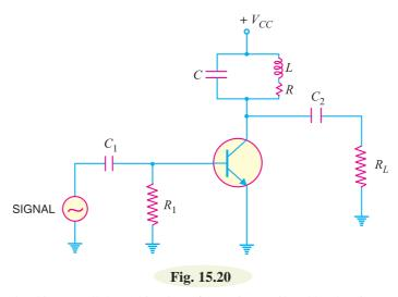
(*ii*) The a.c. load is a parallel combination of capacitor, coil and load resistance  $R_L$  as shown in Fig. 15.21 (*i*). The series resistance R of the inductor can be replaced by its equivalent parallel resistance  $R_p$  as shown in Fig. 15.21 (*ii*) where
