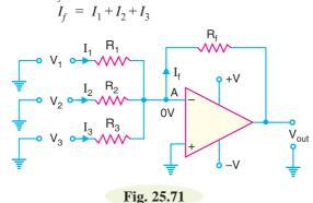
When all the three inputs are applied, the output voltage is Output voltage,  $V_{uut} = -I_c R_c = -R_c (I_1 + I_2 + I_3)$
