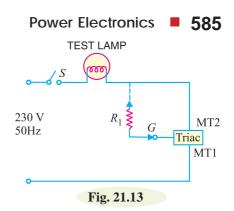
**Example 21.3.** The triac shown in Fig. 21.14 can be triggered by the gate triggering voltage  $V_{GT} = \pm 2V$ . How will you trigger the triac by (i) only a positive gate voltage (ii) only a negative gate voltage ?
