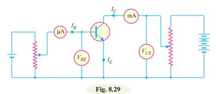
1. Input characteristic. It is the curve between base current  $I_B$  and base-emitter voltage  $V_{BE}$  at constant collector-emitter voltage  $V_{CE}$ .
