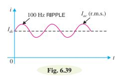
By definition, the effective (*i.e.* r.m.s.) value of total load current is given by :
