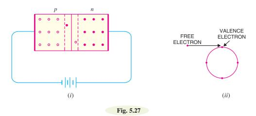
(*ii*) Knee voltage. It is the forward voltage at which the current through the junction starts to increase rapidly.
