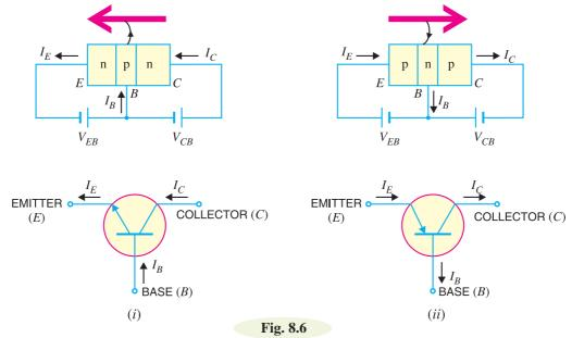
Note that emitter is shown by an arrow which indicates the direction of conventional current flow with forward bias. For *npn* connection, it is clear that conventional current flows out of the emitter as indicated by the outgoing arrow in Fig. 8.6 (*i*). Similarly, for *pnp* connection, the conventional current flows into the emitter as indicated by inward arrow in Fig. 8.6 (*ii*).
