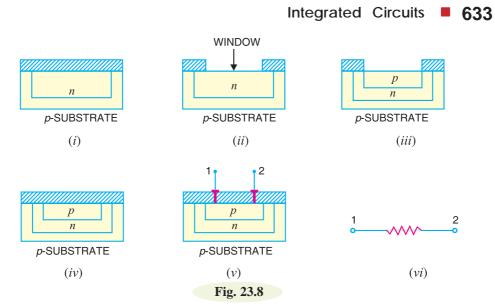
The value of resistor is determined by the material, its length and area of cross-section. The high-resistance resistors are long and narrow while low-resistance resistors are short and of greater cross-section.
