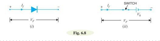
We assume here that *V/I* characteristic of crystal diode is linear.
