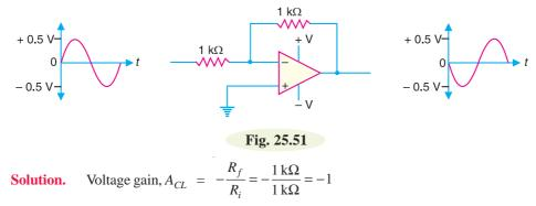
Since the voltage gain of the circuit is –1, the **output will have the same amplitude but with 180**° **phase inversion.**
