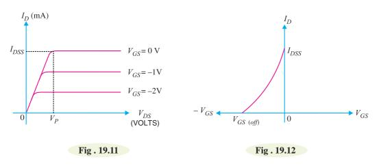
**3.** Gate-source cut off voltage  $V_{GS \text{ (off)}}$ . It is the gate-source voltage where the channel is completely cut off and the drain current becomes zero.
