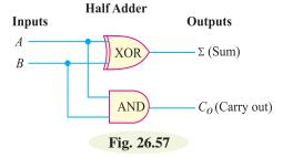
Fig. 26.57. The half adder circuit adds only the LSB column (1s column) in a binary addition problem. The reason is that it has no input for a carry-in.
