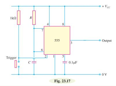
**Example 23.2.** The monostable multivibrator like the one in Fig. 23.17 has the values of  $R = 1.2 k\Omega$  and  $C = 0.1 \mu$ F. Determine the time T for which the circuit is on.
