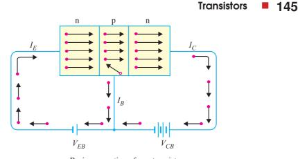
Basic connection of npn transistor
