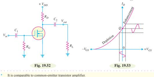
**Operation.** The input signal  $(V_{in})$  is capacitively coupled to the gate terminal. In the absence of the signal, d.c. value of  $V_{GS} = 0$ V. When signal  $(V_{in})$  is applied,  $V_{gs}$  swings above and below its zero value (Q d.c. value of  $V_{GS} = 0$ V), producing a swing in drain current  $I_d$ .
