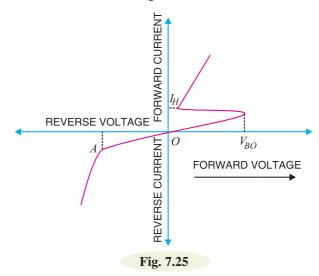
(*ii*) When Shockley diode is reverse biased (*i.e.*, anode is negative *w.r.t.* cathode), diodes  $D_1$  and  $D_3$  would be reverse-biased while diode  $D_2$  would be forward-biased. If reverse voltage is increased sufficiently, the reverse voltage breakdown (point A in Fig. 7.25) of Shockley diode is reached. At this point, diodes  $D_1$  and  $D_3$  would go into reverse-voltage breakdown, the reverse current flowing
