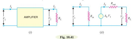
Note that capability of the amplifier to produce voltage gain is represented by the voltage generator  $A_0V_1$ . The voltage gain of the loaded amplifier is  $A_v$ . Clearly,  $A_v$  will be less than  $A_0$  due to voltage drop in  $R_{out}$ .
