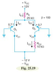
**Solution.** For the *pnp* transistor, the emitter voltage  $(V_E)$  is a diode drop above the base voltage. Therefore,  $V_E = +$  0.7 V.
