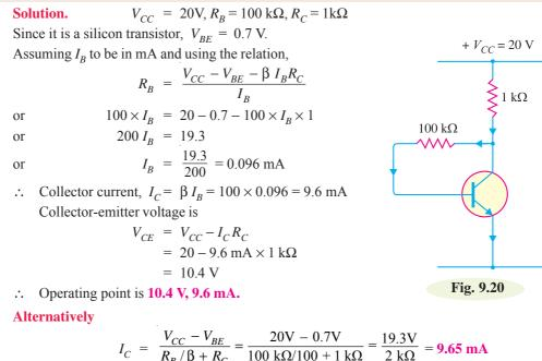
$$I_C = \frac{V_{CC} - V_{BE}}{R_B / \beta + R_C} = \frac{20V - 0.7V}{100 \text{ k}\Omega / 100 + 1 \text{ k}\Omega} = \frac{19.3V}{2 \text{ k}\Omega} = 9.65 \text{ mA}$$
