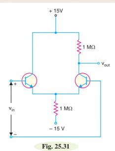
**Solution.** The ideal tail current,  $I_E = V_{EE}/R_E = 15V/1M\Omega = 15 \,\mu$ A. Therefore, d.c. emitter current in each transistor =  $I_{E1} = I_{E2} = I_E/2 = 15 \,\mu$ A/2 = 7.5  $\mu$ A.
