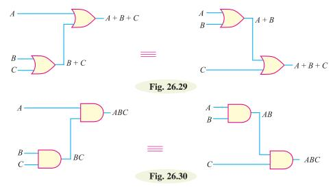
Figure 26.29 illustrates the associative law as applied to the OR gate, while Fig. 26.30 illustrates the associative law as applied to an AND gate.
