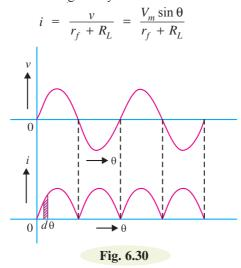
**d.c. output power.** The output current is pulsating direct current. Therefore, in order to find the d.c. power, average current has to be found out. From the elementary knowledge of electrical engineering,
