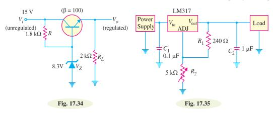
5. If  $R_2$  in Fig. 17.35 is adjusted to 1.68 k $\Omega$ , determine the regulated d.c.output voltage for the LM 317. [10 V]
