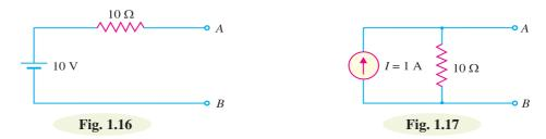
(iii) The equivalent current source is a source of 1 A in parallel with a resistance of 10  $\Omega$  as shown in Fig. 1.17.
