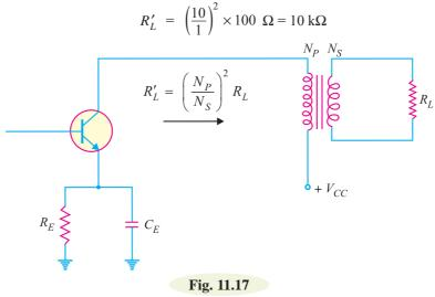
\* There are hundreds of turns of primary and secondary. These turns will multiply an induced e.m.f. from nearby power wiring. As the transformer is connected in the base circuit, therefore, the induced hum voltage will appear in amplified form in the output.
