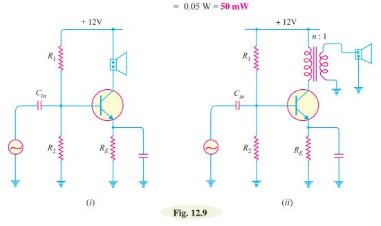
Therefore, when loudspeaker is directly connected in the collector, only 50 mW of power is transferred to the loudspeaker.
