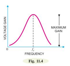
The performance of an amplifier depends to a considerable extent upon its frequency response. While designing an amplifier, appropriate steps must be taken to ensure that gain is essentially uniform over some specified frequency range. For instance, in case of an audio amplifier, which is used to amplify speech or music, it is necessary that all the frequencies in the sound spectrum (*i.e.* 20 Hz to 20 kHz) should be uniformly amplified otherwise speaker will give a distorted sound output.
