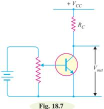
minimum current (called collector leakage current) flows through the load. In other words, a switching transistor has two states viz. (*i*) ON state or when collector saturation current flows through the load (*ii*) OFF state or when collector leakage current flows through the load. In the discussion that follows transistor means the switching transistor.
