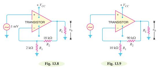
**Example 13.12.** Fig. 13.9 shows the circuit of a negative voltage feedback amplifier. If without feedback,  $A_v = 10,000$ ,  $Z_{in} = 10 k\Omega$ ,  $Z_{out} = 100 \Omega$ , find :
