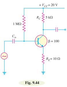
collector current increases and collector-emitter voltage decreases. Moreover, during the positive half cycle of the signal (*i.e.* from 0 to  $\pi$  rad.), the operating point moves from 20  $\mu$ A to 20 + 10 = 30  $\mu$ A and then back again *i.e.* operating point follows the path Q to C and back to Q on the load line.
