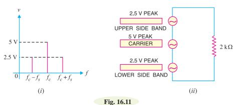
(iii) Power delivered by upper sideband component is
