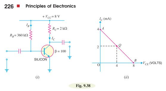
Since  $V_{CE}$  is nearly one-half of  $V_{CC}$ , the amplifier circuit is midpoint biased.
