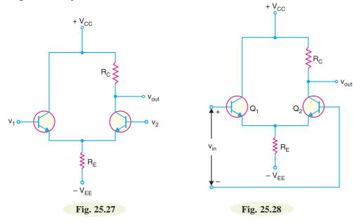
If you look at the differential amplifier circuit in Fig. 25.27, it responds to the difference between the voltages at the two input terminals. In other words, *DA* responds to  $v_{in} (= v_1 - v_2)$ . Therefore, the circuit shown in Fig. 25.27 can be drawn as shown in Fig. 25.28.
