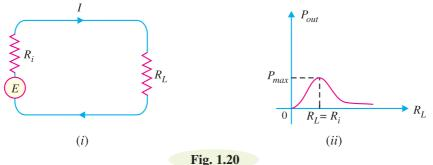
For a given source, generated voltage E and internal resistance  $R_i$  are constant. Therefore, power delivered to the load depends upon  $R_L$ . In order to find the value of  $R_L$  for which the value of P is maximum, it is necessary to differentiate eq. (i) w.r.t.  $R_L$  and set the result equal to zero.
