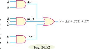
this form is always only a *two-level* gate network *i.e.* the maximum number of gates through which a signal must pass in going form input to output is two (excluding inversions, but these can also be worked in).
