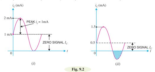
(*ii*) **Proper minimum base-emitter voltage.** In order to achieve faithful amplification, the base-emitter voltage  $(V_{BE})$  should not fall below 0.5V for germanium transistors and 0.7V for *Si* transistors at any instant.
