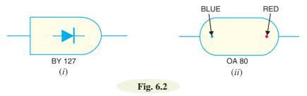
(*ii*) Sometimes, red and blue marks are used on the body of the crystal diode. Red mark denotes arrow whereas blue mark indicates bar *e.g. OA80* crystal diode [See Fig. 6.2 (*ii*)].
