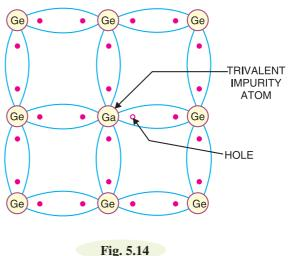
electron to contribute as all its three valence electrons are already engaged in the co-valent bonds with neighbouring germanium atoms. In other words, fourth bond is incomplete; being short of one electron. This missing electron is called a *hole*. Therefore, for each gallium atom added, one hole is created. A small amount of gallium provides millions of holes.
