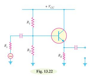
**Example 13.23.** Determine the output impedance of the emitter follower shown in Fig. 13.23. Given that  $r'_e = 20 \Omega$ .
