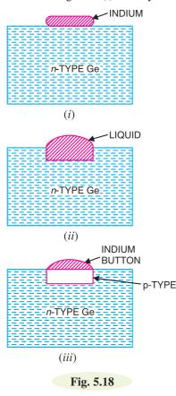
some of the germanium melt to form a small puddle of molten germanium-indium mixture as shown in Fig. 5.18 (*ii*). The temperature is then lowered and puddle begins to solidify. Under proper conditions, the atoms of indium impurity will be suitably adjusted in the germanium slab to form a single crystal. The addition of indium overcomes the excess of electrons in the *n*-type germanium to such an extent that it creates a *p*-type region.
