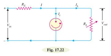
**Operation.** The glow tube will maintain constant voltage across the load inspite of the changes in load current or input voltage. Now, should the load decrease, the output voltage would tend to
