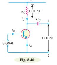
From exps. (i) and (ii), it is clear that magnitude of output is the same whether we take output across collector load or terminals 1 and 2. The minus sign in exp. (ii) simply indicates the phase reversal. The second method of taking output is used in multistages of amplification.
