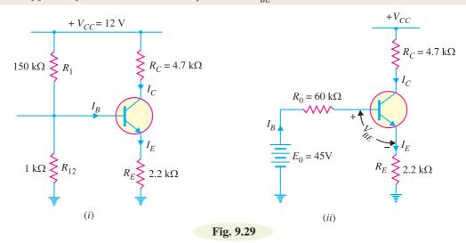
Solution. Fig. 9.29 (i) shows the circuit of potential divider bias whereas Fig. 9.29 (ii) shows it with potential divider circuit replaced by Thevenin's equivalent circuit.
