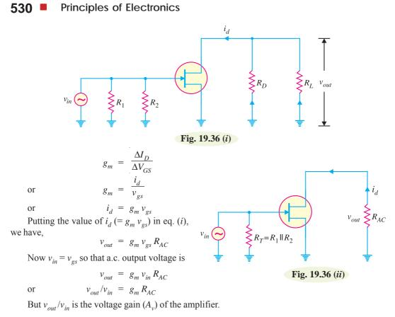
:. Voltage gain,  $A_v = g_m R_{AC}$  ... for loaded amplifier
