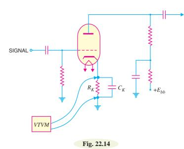
(i) d.c. voltage measurements. A VTVM can accurately measure the d.c. voltages in an electronic circuit. The d.c. voltage to be measured is applied at the input (*i.e.* grid of  $V_1$ ) terminals in such a way that grid of the input valve  $V_1$  is always negative. Fig. 22.14 shows the circuit of an amplifier stage and measurement of d.c. voltage across cathode resistor  $R_{K}$ .
