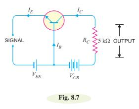
shown. This d.c. voltage is known as bias voltage and its magnitude is such that it always keeps the input circuit forward biased regardless of the polarity of the signal.
