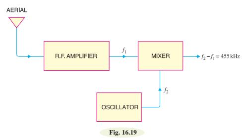
The production of fixed intermediate frequency (455 kHz) is the salient feature of superhetrodyne circuit. At this fixed intermediate frequency, the amplifier circuits operate with maximum stability, selectivity and sensitivity. As the conversion of incoming radio frequency to the intermediate frequency is achieved by *heterodyning* or beating the local oscillator against radio frequency, therefore, this circuit is called \*superhetrodyne circuit.
