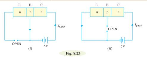
Solution. When the emitter circuit is open [See Fig. 8.23 (i)], the collector-base junction is reverse biased. A small leakage current  $I_{CBO}$  flows due to minority carriers.
