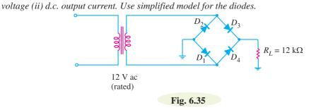
**Solution.** The conditions of the problem suggest that the a.c voltage across transformer secondary is 12V r.m.s.
