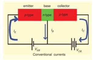
current almost entirely flows in the collector circuit. Therefore, a transistor transfers the input signal current from a low-resistance circuit to a high-resistance circuit. This is the key factor responsible for
