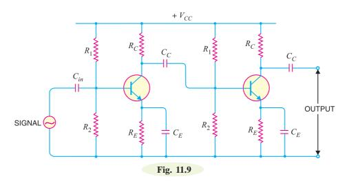
**Operation**. When a.c. signal is applied to the base of the first transistor, it appears in the amplified form across its collector load  $R_C$ . The amplified signal developed across  $R_C$  is given to base of next stage through coupling capacitor  $C_C$ . The second stage does further amplification of the signal. In this way, the *cascaded* (one after another) stages amplify the signal and the overall gain is considerably increased.
