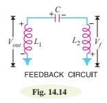
**Feedback fraction m**<sub>v</sub>. In Hartley oscillator, the feedback voltage is across  $L_2$  and output voltage is across  $L_1$ .
