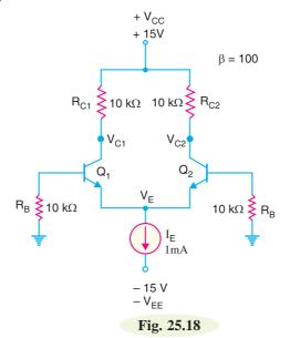
**Solution.** In this circuit, the current  $I_E$  is given by the current source. Ignoring base current, the potential at each emitter is  $V_E = -0.7$  V.
