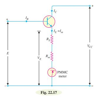
**Operation.** The voltage *E* to be measured is applied between base and emitter of the transistor and causes a base current  $I_B$  to flow through the base circuit. Therefore, collector current  $I_C = \beta I_B$  where  $\beta$  is the current amplification factor of the transistor. Since  $I_E \simeq I_C$  and the meter is connected
