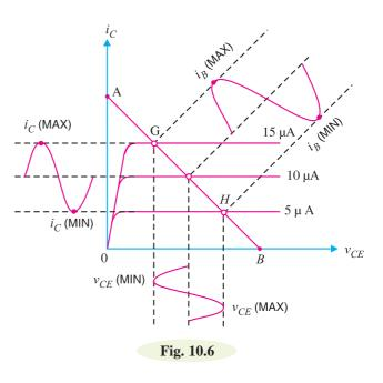
put and output voltages are in *phase opposition* or equivalently, the transistor is said to produce a 180° phase reversal of output voltage w.r.t. signal voltage.
