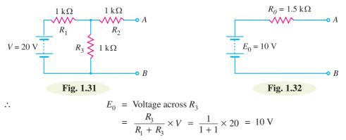
The Thevenin's resistance  $R_0$  is the resistance measured between terminals A and B with no load (i.e. open at terminals A and B) and voltage source replaced by a short circuit.
