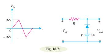
6. Determine the output waveform for the clipper network shown in Fig. 18.71.
