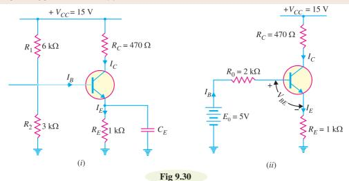
**Solution.** Fig. 9.30 (*i*) shows the circuit of potential divider bias whereas Fig. 9.30 (*ii*) shows it with potential divider circuit replaced by Thevenin's equivalent circuit.
