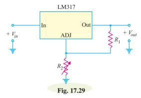
The *LM* 317 is a three-terminal positive adjustable voltage regulator and can supply 1.5 A of load current over an adjustable output range of 1.25V to 37V. Fig. 17.29 shows an unregulated power supply driving an *LM* 317 circuit. The data sheet of an *LM* 317 gives the following formula for the output voltage :
