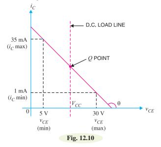
(*i*) The zero signal collector current is approximately half-way between the maximum and minimum values of collector current *i.e.*
