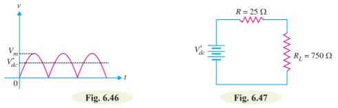
For d.c. component  $V'_{dc}$ , the choke resistance is in series with the load as shown in Fig. 6.47.
