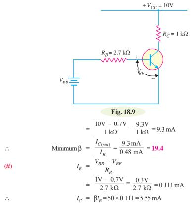
Since the collector current is less than saturation current (= 9.3 mA), the transistor will not be saturated.
