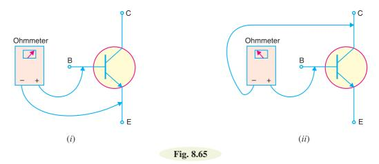
(*ii*) The reverse biased collector-base junction (again reverse biased by internal supply) should be checked as shown in Fig. 8.65 (*ii*). If the reading of the ohmmeter is 100 k $\Omega$  or higher, the transistor is good. If the ohmmeter registers a small resistance, the transistor is faulty and requires replacement.
