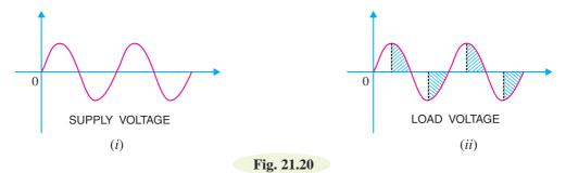
The firing of triac can be controlled upto a maximum of 180°. In this way, we can provide a continuous control of load voltage from practically zero to full *r.m.s.* value.
