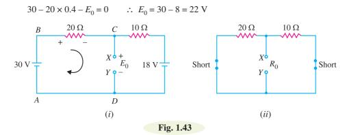
To find  $R_0$ , we short both voltage sources as shown in Fig. 1.43 (*ii*). Notice that 10  $\Omega$  and 20  $\Omega$  resistors are then in parallel.
