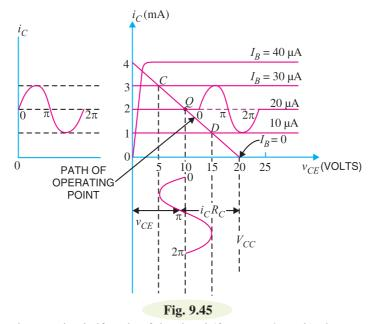
(*ii*) During the negative half-cycle of the signal (from  $\pi$  to  $2\pi$  rad.), the operating point goes from 20  $\mu$ A to 20 – 10 = 10  $\mu$ A and then back again *i.e.* the operating point follows the path Q to D and back to Q on the load line.
