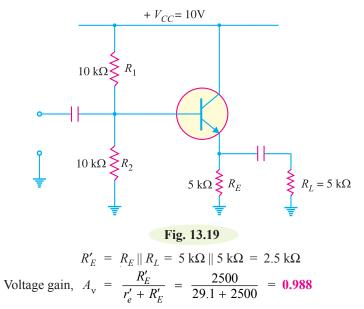
**Comments.** This is the same example as example 13.20 except that load is added. Note the loading effect on the voltage gain of an emitter follower. When load is added to the emitter follower, the voltage gain drops from 0.994 to 0.988. This is really a small change. On the other hand, when a CE amplifier is loaded, there is drastic change in voltage gain. This is yet another difference between the emitter follower and CE amplifier.
