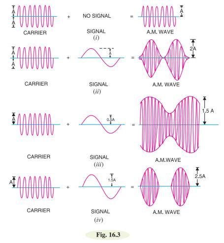
(*iii*) When the signal amplitude is one-half the carrier amplitude as shown in Fig. 16.3 (*iii*), the amplitude of carrier wave varies between 1.5 A and 0.5 A.
