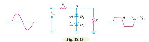
**Solution.** The symmetrical zener clipper uses two zener diodes that are connected as shown in Fig. 18.43. When the input is positive,  $D_1$  is forward biased and  $D_2$  is reverse biased (assuming that the value of  $V_{in}$  is high enough to turn both diodes ON). When both diodes are conducting, the voltage from point A to ground will be equal to the sum of  $V_{Z2}$  and the forward voltage drop of  $D_1$  *i.e.*,  $V_{F1} = 0.7$ V.
