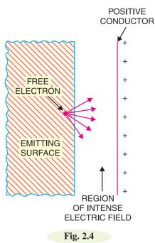
Very intense electric field is required to produce field emission. Usually, a voltage of the order of a million volts per centimetre distance between the emitting surface and the positive conductor is necessary to cause field emission. Field emission can be obtained at temperatures much lower (*e.g.* room temperature) than required for thermionic emission and, therefore, it is also sometimes called *cold cathode emission* or *auto- electronic emission*.
