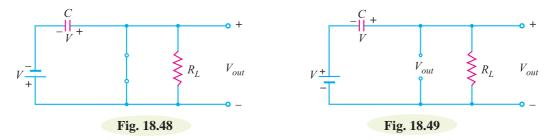
(*ii*) When the input switches to +V state (*i.e.*, positive half-cycle), the diode is reverse biased and behaves as an open as shown in Fig. 18.49. Since the discharging time constant (=  $CR_L$ ) is much greater than the time period of the input signal, the capacitor remains almost fully charged to V volts during the off time of the diode. Referring to Fig. 18.49 and applying Kirchhoff 's voltage law to the input loop, we have,
