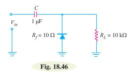
\*Charging time constant,  $\tau = R_f C = (10 \ \Omega) \times (10^{-6} \text{ F}) = 10 \ \mu\text{s}$ Total charging time,  $\tau_C = **5R_f C = 5 \times 10 = 50 \ \mu\text{s}$
