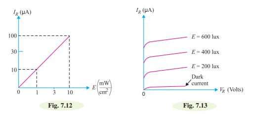
(ii) Reverse voltage-Reverse current curve. Fig. 7.13 shows the graph between reverse current  $(I_R)$  and reverse voltage  $(V_R)$  for various illumination levels. It is clear that for a given
