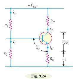
**Circuit analysis.** Suppose that the current flowing through resistance  $R_1$  is  $I_1$ . As base current  $I_B$  is very small, therefore, it can be assumed with reasonable accuracy that current flowing through  $R_2$ is also  $I_1$ .
