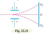
the spot of light will be deflected upwards (point  $O_1$ ). The spot of light will be deflected downwards (point  $O_2$ ) if the potential on the plates is reversed. Similarly, the spot of light can be moved horizontally by applying voltage across the horizontal plates.
