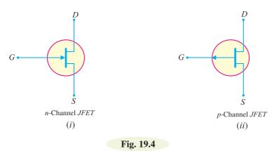
as channel and source (S) and drain (D) connected to this line. If the channel is *n*-type, the arrow on the gate points towards the channel as shown in Fig. 19.4 (*i*). However, for *p*-type channel, the arrow on the gate points from channel to gate [See Fig. 19.4 (*ii*)].
