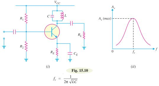
At the resonant frequency, the impedance of the parallel resonant circuit is very high and is purely resistive. Therefore, when the circuit is tuned to resonant frequency, the voltage across  $R_L$  is maximum. In other words, the voltage gain is maximum at  $f_r$ . However, above and below the resonant frequency, the voltage gain decreases rapidly. The higher the Q of the circuit, the faster the gain drops off on either side of resonance [See Fig. 15.10 (*ii*)].
