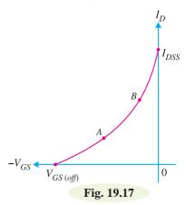
$$g_m = g_{mo} \left( 1 - \frac{V_{GS}}{V_{GS \ (off)}} \right)$$
