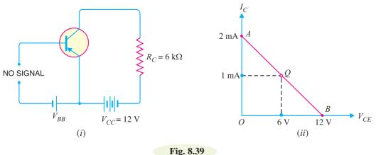
Zero signal collector-emitter voltage is
