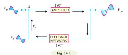
feedback. Remember that a positive feedback amplifier is one that produces a feedback voltage  $(V_f)$  that *is in phase* with the original input signal. As you can see, this condition is met in the circuit shown in Fig. 14.5. A phase shift of 180° is produced by the amplifier and a further phase shift of 180° is introduced by feedback network. Consequently, the signal is shifted by 360° and fed to the input *i.e.*, feedback voltage is in phase with the input signal.
