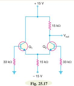
**Solution.** Tail current,  $I_E = \frac{V_{EE} - V_{BE}}{R_E} = \frac{(15 - 0.7)V}{15 \text{ k}\Omega} = 0.953 \text{ mA}$
