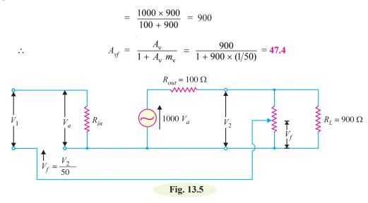
**Example 13.10.** An amplifier is required with a voltage gain of 100 which does not vary by more than 1%. If it is to use negative feedback with a basic amplifier the voltage gain of which can vary by 20%, determine the minimum voltage gain required and the feedback factor.
