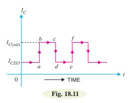
Fig. 18.11. This condition will prevail for a time (*bc* in this case) determined by circuit conditions. After this time, transistor  $Q_2$  is cut off and  $Q_1$  is turned ON. The collector current in  $Q_2$  is now  $I_{CEO}$  as shown. The circuit will stay in this condition for a time *de*. Again  $Q_2$  is turned ON and  $Q_1$  is driven to cut off. In this way, the output will be a square wave.
