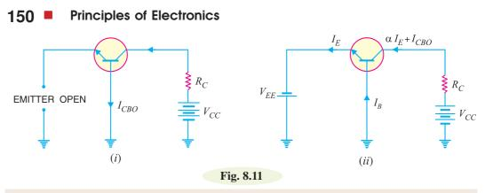
**Example 8.2.** In a common base connection,  $I_E = ImA$ ,  $I_C = 0.95mA$ . Calculate the value of  $I_B$ . **Solution.** Using the relation,  $I_E = I_B + I_C$ or  $1 = I_B + 0.95$  $\therefore \qquad I_B = 1 - 0.95 = 0.05 \text{ mA}$
