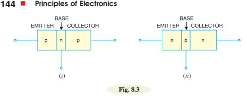
(*iii*) The transistor has two *pn* junctions *i.e.* it is like two diodes. The junction between emitter and base may be called *emitter-base diode* or simply the *emitter diode*. The junction between the base and collector may be called *collector-base diode* or simply *collector diode*.
