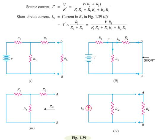
To find  $R_N$ , remove the load  $R_L$  and replace the voltage source by a short circuit because its resistance is assumed zero [See Fig. 1.39 (*iii*)].
