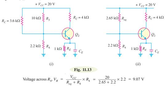
Thus the biasing potential of second stage is drastically changed. The 9.07 V at the base of  $Q_2$  would undoubtedly cause the transistor to saturate and the device would be rendered useless as an amplifier. This example explains the importance of dc isolation in a multistage amplifier. The use of coupling capacitor allows each amplifier stage to maintain its independent biasing potential while allowing the ac output from one stage to pass on to the next stage.
