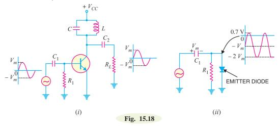
(*ii*) When an a.c. signal is applied, *clamping action* takes place as shown in Fig. 15.18 (*ii*). The voltage across the emitter diode varies between + 0.7 V (during positive peaks of input signal) to about  $-2V_m$  (during negative peaks of input signal). This means that conduction of the transistor occurs only for a short period during positive peaks of the signal. This results in the pulsed output *i.e.* collector current waveform is a train of narrow pulses (Refer back to Fig. 15.17).
