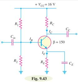
**Solution.** We are given  $V_{CC}$ ,  $\beta$  and the operating point. It is desired to find the component values. For good design, voltage across  $R_E$  (*i.e.*,  $V_E$ ) should be one-tenth of  $V_{CC}$  *i.e.*
