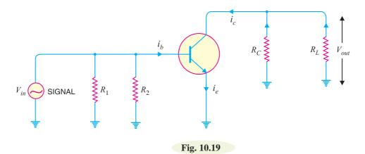
It is clear that as far as a.c. signal is concerned, load  $R_C$  appears in parallel with  $R_L$ . Therefore, effective load for a.c. is given by :
