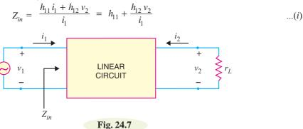
Now,  $i_2 = h_{21} i_1 + h_{22} v_2$  in terms of *h* parameters. Further from Fig. 24.7, it is clear that  $i_2 = -v_2/r_L$ . The minus sign is used here because the actual load current is opposite to the direction of  $i_2$ .
