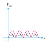
**Peak inverse voltage.** Suppose  $V_m$  is the maximum voltage across the half secondary winding. Fig. 6.25 shows the circuit at the instant secondary voltage reaches its maximum value in the positive direction. At this instant, diode  $D_1$  is conducting while diode  $D_2$  is non-conducting. Therefore, whole of the secondary voltage appears across the non-conducting diode. Consequently, the peak inverse voltage is twice the maximum voltage across the half-secondary winding *i.e.*
