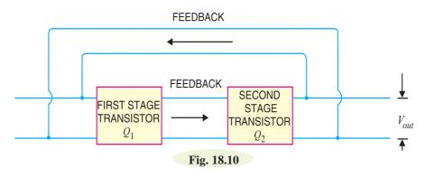
A multivibrator is a switching circuit which depends for operation on positive feedback. It is basically a two-stage amplifier with output of one fedback to the input of the other as shown in Fig. 18.10.
