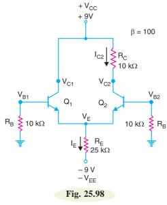
$[V_E = -0.7 \text{ V}; I_E = 0.332 \text{ mA}; I_{E1} = I_{E2} = 0.166 \text{ mA}; I_{C1} = I_{C2} = 0.166 \text{ mA}; I_{B1} = I_{B2} = 1.66 \mu\text{A}; V_{C1} = 9 \text{ V}; V_{C2} = 7.34 \text{ V}]$
