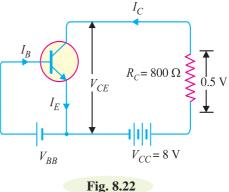
**Example 8.13.** An n-p-n transistor at room temperature has its emitter disconnected. A voltage of 5V is applied between collector and base. With collector positive, a current of 0.2  $\mu$ A flows. When the base is disconnected and the same voltage is applied between collector and emitter, the current is found to be 20  $\mu$ A. Find  $\alpha$ ,  $I_E$  and  $I_B$  when collector current is 1mA.
