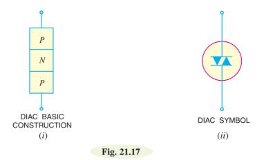
The diac can be constructed in either npn or pnp form. Fig. 21.17 (*i*) shows the basic structure of a diac in pnp form. The two leads are connected to p-regions of silicon separated by an n-region. The structure of diac is very much similar to that of a transistor. However, there are several imporant differences:
