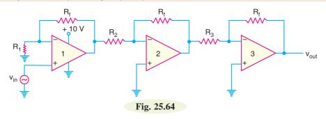
**Solution.** Designing the above OP-amp circuit means to find the values of  $R_1$ ,  $R_2$  and  $R_3$ . The first stage gain is +10 so that this stage operates as noninverting amplifier.
