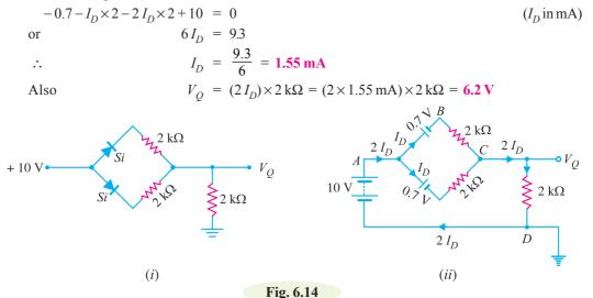
**Example 6.8.** Determine current through each diode in the circuit shown in Fig. 6.15 (i). Use simplified model. Assume diodes to be similar.
