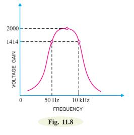
*Comments.* As bandwidth of the amplifier is 50 Hz to 10 kHz, therefore, it will amplify the signal frequencies lying in this range without any
