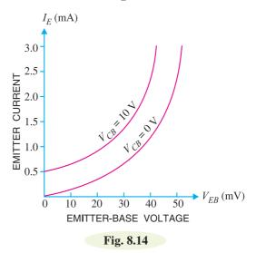
change in emitter current ( $\Delta I_E$ ) at constant collector-base voltage ( $V_{CB}$ ) *i.e.*
