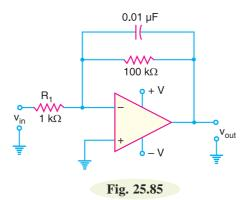
Solution. The critical frequency for the integrator circuit shown in Fig. 25.85 is given by;
