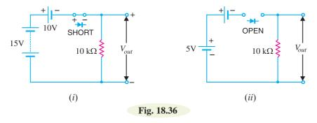
For any value of  $V_{in} < 10$ V, the ideal diode is reverse biased. Therefore, circuit current is zero and hence  $V_{out} = 0$ . For example, with  $V_{in} = 5$ V [See Fig. 18.36 (*ii*)],  $V_{out} = 0$  and  $V_d$  (drop across diode) = 5V
