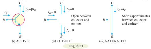
Note. When the transistor is in the active state,  $I_C = \beta I_B$ . Therefore, a transistor acts as an amplifier when operating in the active state. Amplification means *linear amplification*. In fact, small signal amplifiers are the most common *linear devices*.
