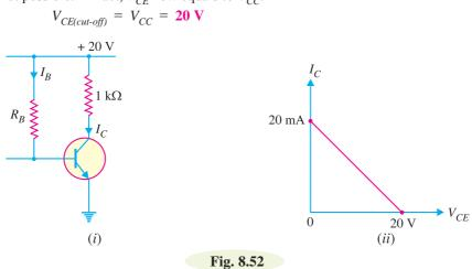
Figure 8.52 (*ii*) shows the saturation and cut off points. Incidentally, they are end points of the d.c. load line.
