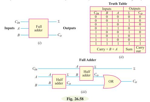
The full adder has three inputs :  $C_{in}$ , A and B. These three inputs must be added to get the  $\Sigma$  and  $C_o$  outputs. Fig. 26.58 (*ii*) shows the truth table for a full adder. It shows all the possible combinations of A, B and  $C_{in}$ . The full adder is used for binary addition in all places except the 1s place which means 2s, 4s, 8s etc.
