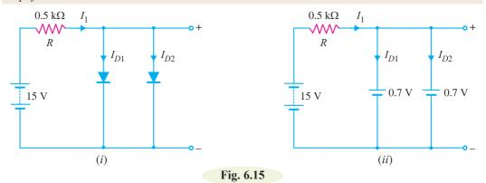
**Solution.** The applied voltage forward biases each diode so that they conduct current in the same direction. Fig. 6.15 (*ii*) shows the equivalent circuit using simplified model. Referring to Fig. 6.15 (*ii*),
