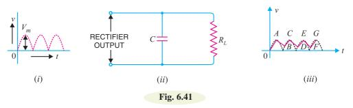
The capacitor filter circuit is extremely popular because of its low cost, small size, little weight and good characteristics. For small load currents (say upto 50 mA), this type of filter is preferred. It is commonly used in transistor radio battery eliminators.
