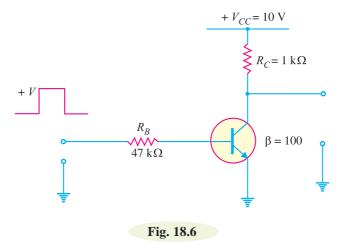
Hence in order to saturate the transistor, we require + 5.4 V.
