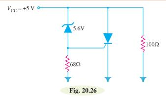
Solution. The breakdown voltage of the zener is 5.6V. To turn on the SCR, the voltage across  $68\Omega$  has to be equal to  $V_T (= 0.7 \text{V})$ .
