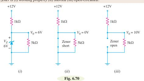
**Solution.** Zener diodes cannot be tested individually with a multimeter. It is because multimeters usually do not have enough input voltage to put the zener into breakdown region.
