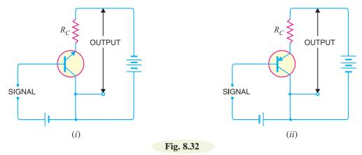
(*i*) Current amplification factor  $\gamma$ . In common collector circuit, input current is the base current  $I_B$  and output current is the emitter current  $I_E$ . Therefore, current amplification in this circuit arrangement can be defined as under :
