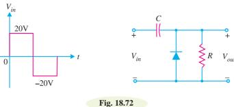
7. Determine the output waveform for the clamper network shown in Fig. 18.72.
