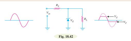
**Solution.** The *zener shunt clipper* uses a zener diode in place of the ordinary diode. The zener shunt clipper uses both the forward and reverse characteristics of the zener diode. Thus when the zener diode is forward biased, this clipper acts just like the standard shunt clipper.
