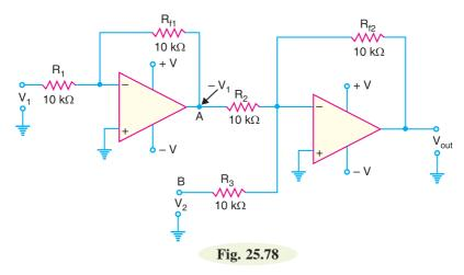
The voltage  $V_1$  is applied to a standard inverting amplifier that has *unity gain*. Because of this, the output from the inverting amplifier will be equal to  $-V_1$ . This output is then applied to the summing amplifier (also having unity gain) along with  $V_2$ . Thus output from second *OP*-amp is given by;
