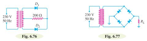
7. In Fig. 6.76, the maximum voltage across half of secondary winding is 50 V. Find (*i*) the average load voltage (*ii*) peak inverse voltage (*iii*) output frequency. Assume the diodes to be ideal.
