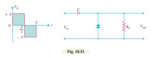
(ii) When the input switches to -V state (i.e., negative half-cycle), the diode is reverse biased
