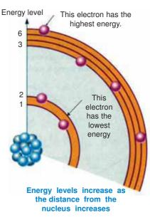
The number and arrangement of protons, neutrons and electrons.
