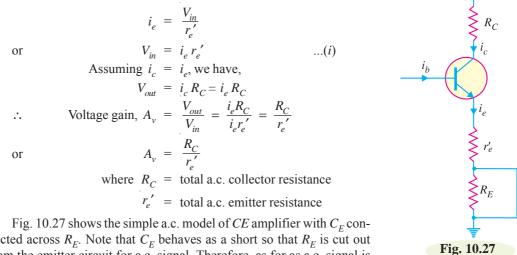
nected across  $R_E$ . Note that  $C_E$  behaves as a short so that  $R_E$  is cut out from the emitter circuit for a.c. signal. Therefore, as for as a.c. signal is concerned, the total a.c. emitter resistance is  $r_e'$ .
