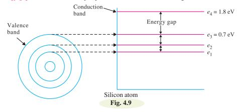
(e.g. heat) equal to the energy difference of the orbits must be supplied. For example, the valence band is shown to have an energy level of 0.7 eV. The conduction band is shown to have an energy level of 1.8 eV. Thus for an electron to jump from the valence band to the conduction band, an energy = 1.8 - 0.7 = 1.1 eV must be supplied. As you will see, the energy band description of substances is very important in understanding many fields of science and engineering including electronics.
