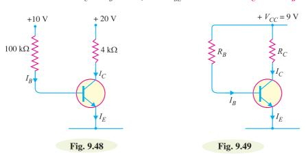
4. A transistor amplifier is biased with feedback resistor  $R_B$  of 100 kΩ. If  $V_{CC} = 25$  V,  $R_C = 1$  kΩ and  $\beta = 200$ , find the values of zero signal  $I_C$  and  $V_{CE}$ .  $[I_C = 16.2$ mA,  $V_{CE} = 8.8$ V]
