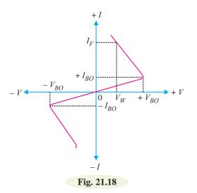
Diacs are used primarily for triggering of triacs in adjustable phase control of a.c. mains power. Some of the circuit applications of diac are (*i*) light dimming (*ii*) heat control and (*iii*) universal motor speed control.
