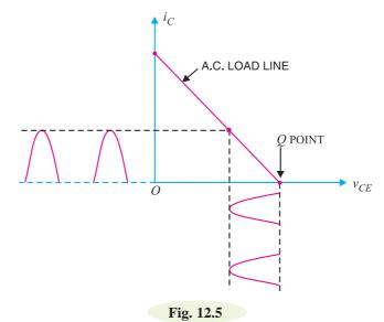
In class *C* amplifier, the base is given some negative bias so that collector current does not flow just when the positive half-cycle of the signal starts. Such amplifiers are never used for power amplification. However, they are used as tuned amplifiers *i.e.* to amplify a narrow band of frequencies near the resonant frequency.
