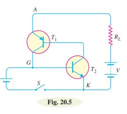
one transistor causes an increase of current in the other transistor. As a result of this action, both
