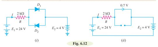
**Solution.** The conditions of the problem suggest that diode  $D_1$  is forward biased and diode  $D_2$  is reverse biased. We can, therefore, consider the branch containing diode  $D_2$  as open as shown in Fig. 6.12 (*ii*). Further, diode  $D_1$  can be replaced by its simplified equivalent circuit.
