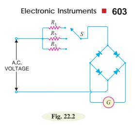
a.c. position. This puts the circuit shown in Fig. 22.2 in action. By throwing the range selector switch S to a suitable position, the given a.c. voltage can be measured. It may be mentioned here that a.c. voltage scale is calibrated in r.m.s. values. Therefore, the meter will give the r.m.s. value of the a.c. voltage under measurement.
