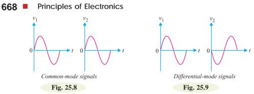
Thus we arrive at a very important conclusion that a differential amplifier will amplify the differential-mode signals while it will reject the common-mode signals.
