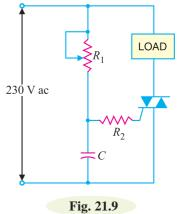
Circuit action. The operation of triac phase control circuit is as under :
