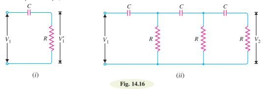
Fig. 14.16 (*ii*) shows the three sections of *RC* network. Each section produces a phase shift of 60°. Consequently, a total phase shift of 180° is produced *i.e.* voltage  $V_2$  leads the voltage  $V_1$  by 180°.
