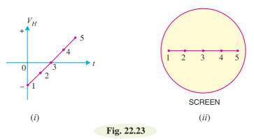
In order that the beam moves from left to right at a uniform rate, a voltage that varies linearly with time should be applied to the horizontal plates. This condition is exactly met in the saw tooth wave shown in Fig. 22.23 (*i*).
