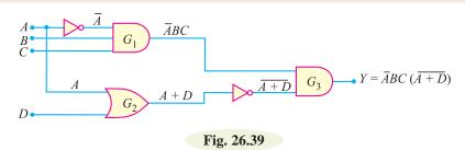
**Solution.** There are two AND gates (viz.  $G_1$  and  $G_3$ ) and one OR gate ( $G_2$ ). Also the circuit has two inverters. The input A is fed to  $G_1$  through the inverter. Therefore,  $\overline{A}$ , B and C are ANDed by  $G_1$ to produce an output of A BC. The input A is ORed with D by  $G_2$  to produce an output of (A + D). The inputs  $\overline{ABC}$  and  $(\overline{A+D})$  to  $G_3$  are ANDed to produce the final output :
