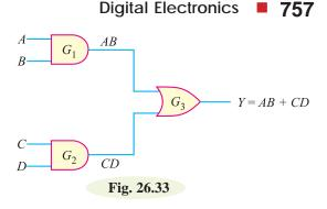
(*ii*) Fig. 26.34 shows a logic circuit consisting of two AND gates and one OR gate. There are four (*A*, *B*, *C* and *D*) input variables.
