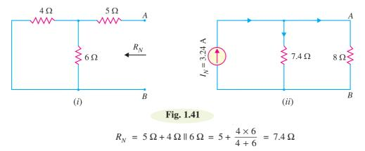
The Norton's equivalent circuit behind terminals *AB* is  $I_N$  (= 3.24 A) in parallel with  $R_N$  (= 7.4  $\Omega$ ). When load (*i.e.*, 8  $\Omega$ ) is connected across terminals *AB*, the circuit becomes as shown in Fig. 1.41 (*ii*). The current source is supplying current to two resistors 7.4  $\Omega$  and 8  $\Omega$  in parallel.
