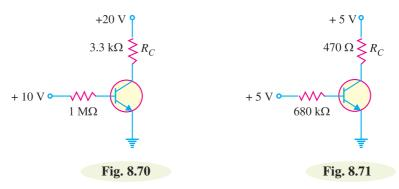
9. If the collector resistance  $R_C$  in Fig. 8.70 is reduced to 1 k $\Omega$ , what happens to the d.c. load line ?
