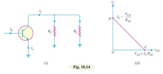
Maximum collector current =  $I_C + \frac{V_{CE}}{R_{AC}}$ where  $R_{AC} = R_C || R_L = \frac{R_C R_L}{R_C + R_L}$ This locates the point *D* of a.c. load line on the collector-current axis. By joining points *C* and *D*,
