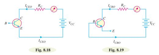
(ii) Circuit for  $I_{CBO}$  test. Fig. 8.19 shows the circuit for measuring  $I_{CBO}$ . Since the emitter is open ( $I_E = 0$ ), there is a small current from collector to base. This is called  $I_{CBO}$  (collector-to-base current with emitter open). This current is due to the movement of minority carriers across basecollector junction. The value of  $I_{CBO}$  is also small. If in measurement,  $I_{CBO}$  is excessive, then there is a possibility that collector-base is shorted.
