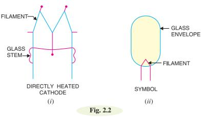
The directly heated cathode is more efficient in converting heating power into thermionic emission. Therefore, it is generally used in power tubes that need large amounts of emission and in small tubes operated from batteries where efficiency and quick heating are important. The principal limitation of this type of cathode is that any variation in heater voltage affects the electron emission and thus produces *hum* in the circuit.
