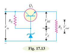
(i) If the output voltage decreases, the increased base-emitter voltage causes transistor  $Q_1$  to conduct more, thereby raising the output voltage. As a result, the output voltage is maintained at a constant level.
