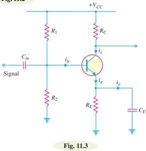
is greatly reduced. Note that  $C_{in}$  is the coupling capacitor in this circuit.
