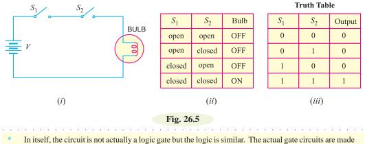
with diodes and transistors. In other words, switches  $S_1$  and  $S_2$  are replaced by diodes or transistors.
