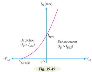
Note that the transconductance curve for the *D-MOSFET* is very similar to the curve for a *JFET*. Because of this similarity, the *JFET* and the *D-MOSFET* have the same transconductance equation *viz*.
