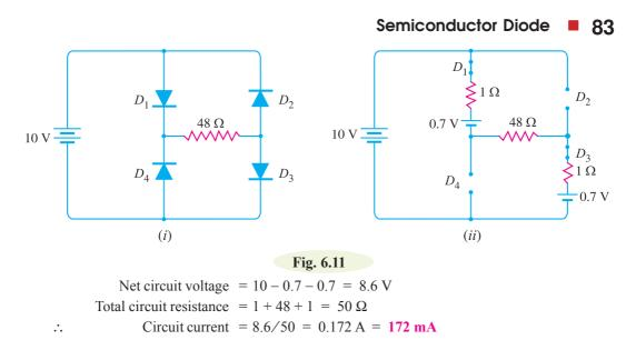
**Example 6.5.** Determine the current I in the circuit shown in Fig. 6.12 (i). Assume the diodes to be of silicon and forward resistance of diodes to be zero.
