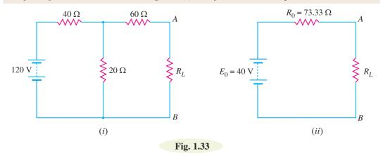
**Solution.** We shall first find Thevenin's equivalent circuit to the left of terminals AB in Fig. 1.33 (*i*).
