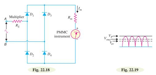
**Operation.** When a.c. voltage to be measured is applied to the circuit, it passes the positive half-cycles of the input and inverts the negative half-cycles.
