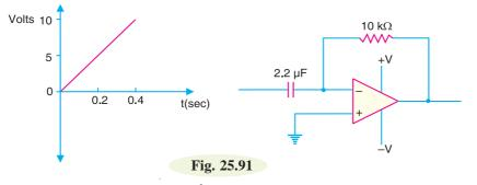
Solution. Output voltage,  $v_o = -RC \frac{dv_i}{dt}$ Now,  $RC = (10 \text{ k}\Omega) \times (2.2 \text{ }\mu\text{F}) = (10^4 \Omega) (2.2 \times 10^{-6} \text{ F}) = 2.2 \times 10^{-2} \text{ s}$ Also,  $\frac{dv_i}{dt} = \frac{(10-0)V}{0.4s} = \frac{10V}{0.4s} = 25 \text{ V/s}$  $\therefore \qquad v_o = -(2.2 \times 10^{-2}) \times 25 = -0.55 \text{ V}$
