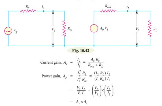
Note. The use of such an equivalent circuit is restricted to the signal quantities only. Further, in drawing the equivalent circuit, it is assumed that exact linear relationship exists between input and output signals *i.e.* the amplifier produces no waveform distortion.
