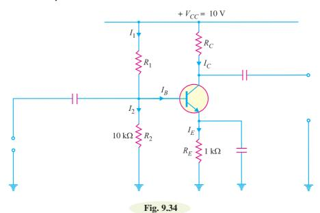
Example 9.29. Fig. 9.35 shows the potential divider method of biasing. What will happen if (i) resistance  $R_2$  is shorted (ii) resistance  $R_2$  is open-circuited (iv) resistance  $R_1$  is open ? (*iii*) resistance  $R_1$  is shorted
