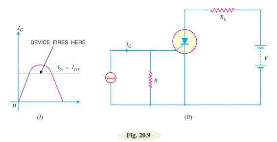
(ii) A.C. trigger circuit. An SCR can also be turned on with positive cycle of a.c. gate current. Fig. 20.9 (ii) shows such a circuit. During the positive half-cycle of the gate current, at some point  $I_G = I_{GT}$ , the device is turned on as shown in Fig. 20.9 (i).
