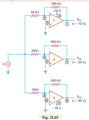
Solution. The resistor component for each stage will be :
