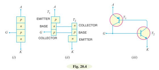
Fig. 20.4 (*ii*). Thus, the equivalent circuit of *SCR* is composed of *pnp* transistor and *npn* transistor connected as shown in Fig. 20.4. (*iii*). It is clear that collector of each transistor is coupled to the base of the other, thereby making a positive feedback loop.
