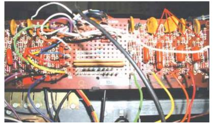
Low voltage differential amplifier for test and measurement applications.
