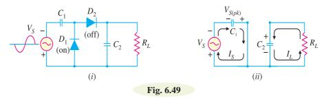
As you can see [See Fig.6.49 (*ii*)],  $C_1$  will charge until voltage across it becomes equal to peak value of source voltage  $[V_{S(pk)}]$ . At the same time,  $C_2$  will be in the process of discharging through the load  $R_L$  (The source of this charge on  $C_2$  will be explained in a moment). Note that in all figures electron flow is shown.
