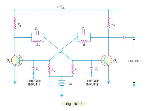
**Operation.** When  $V_{CC}$  is applied, one transistor will start conducting slightly ahead of the other due to some differences in the characteristics of the transistors. This will drive one transistor to
