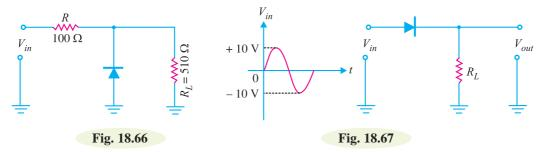
2. In the negative series clipper shown in Fig. 18.67, what is the peak output voltage? [9.3 V]
