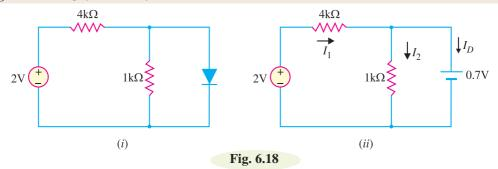
Solution. Let us assume that the diode is ON. Therefore, we can replace the diode with a 0.7V battery as shown in Fig. 6.18 (ii). Referring to Fig. 6.18 (ii), we have,
