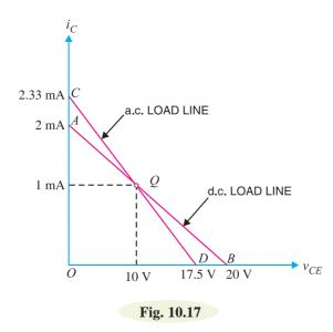
**Comments.** The reader may see that the operating point lies on both a.c. and d.c. load lines. It is not surprising because signal is a.c. and it becomes zero after every half-cycle. When the signal is zero, we have the exact d.c. conditions. Therefore, key point to keep in mind is that the point of intersection of d.c. and a.c. load lines is the operating point Q.
