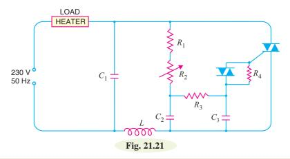
**Example 21.5.** We require a small gate triggering voltage  $V_{GT}$  (say  $\pm 2V$ ) to fire a triac into conduction. How will you raise the trigger level of the triac ?
