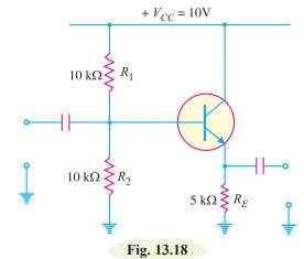
Voltage across  $R_E$ ,  $V_E = V_2 - V_{BE} = 5 - 0.7 = 4.3 \text{ V}$
