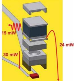
Power Dissipation Channels in a Microfabricated Atomic Clock
