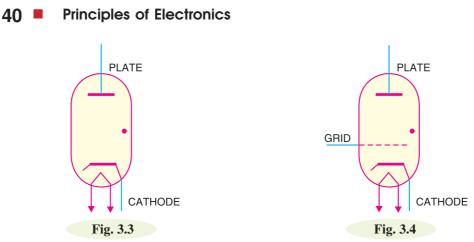
Fig. 3.3 shows the schematic symbol of a hot-cathode gas diode, known as *phanotron* whereas Fig. 3.4 shows the symbol of hot-cathode gas triode, known as *thyratron*.
