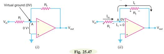
Referring to Fig. 25.47 (*ii*), the current  $I_1$  to the inverting input is zero. Therefore, current  $I_{in}$  flowing through  $R_i$  entirely flows through feedback resistor  $R_f$ . In other words,  $I_f = I_{in}$ .
