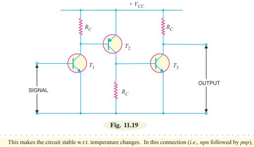
the direction of collector current increase  $\beta$ , when the temperature rises, is opposite for the two transistors. Thus the variation in one transistor tends to cancel that in the other.
