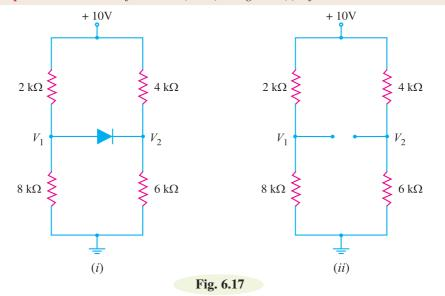
Solution. Let us assume that diode in Fig. 6.17 (i) is OFF i.e. it is reverse biased. The circuit then becomes as shown in Fig. 6.17 (ii). Referring to Fig. 6.17 (ii), we have,
