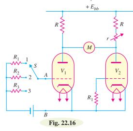
resistance has low value. The imbalance in the plate currents of the two valves will cause a current through the meter M which will directly give the value over the resistance scale of the meter.
