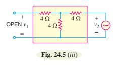
Now the output impedance looking into the output terminals with input terminals open is simply 8  $\Omega$ . Then  $h_{22}$  will be the reciprocal of this *i.e.*
