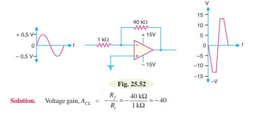
Note that the input signal is the same as in example 25.27 but now the voltage gain is -40 instead of -1. Since the supply voltages are  $\pm$  15 V, the \*saturation occurs at  $\pm$  13 V. Since the output voltage far exceeds the saturation level, the OP-amp will be driven to deep saturation and it will behave as a non-linear amplifier. This means that the output will not have the same shape as input but will clip at the saturation voltage. Note that 180° phase inversion does occur.
