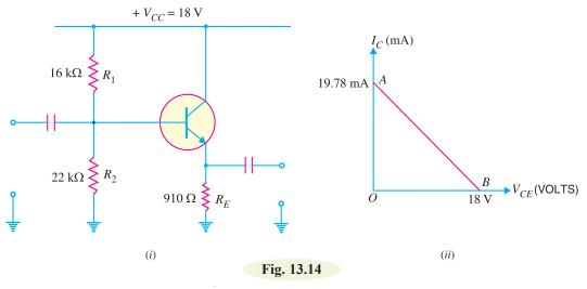
$$I_{C(sat)} = \frac{V_{CC}}{R_E} = \frac{18 \text{ V}}{910 \Omega} = 19.78 \text{ mA}$$
