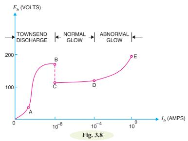
After the glow discharge, the voltage across the tube no longer remains constant. Now, if the supply voltage is raised, not only will the circuit current increase but the voltage across the tube will start to rise again. This stage of conduction (D to E) is known as *abnormal glow*.
