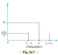
\* From trigonometry, we have the expansion formula : 2 cos A cos B = cos (A + B) + cos (A - B) \*\*  $f_c = \frac{\omega_c}{2\pi}, f_c + f_s = \frac{\omega_c + \omega_s}{2\pi}, f_c - f_s = \frac{\omega_c - \omega_s}{2\pi}$
