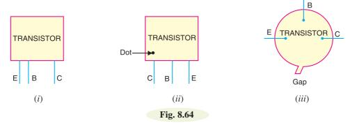
(*ii*) When the leads of a transistor are in the same plane but evenly spaced [See Fig. 8.64 (*ii*)], the central lead is the base, the lead identified by dot is the collector and the remaining lead is the emitter.
