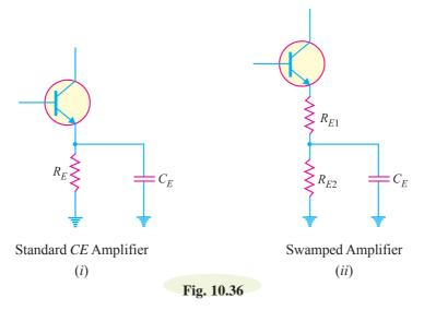
Fig. 10.36 (*i*) shows the emitter leg of a standard *CE* amplifier while Fig. 10.36 (*ii*) shows the emitter leg of swamped amplifier. In swamped amplifier, the resistance  $R_E$  is split into two parts *viz*.  $R_{E1}$  and  $R_{E2}$ . Only  $R_{E2}$  is bypassed by  $C_E$  while  $R_{E1}$  is not.
