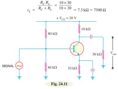
(i) The input impedance looking into the base of transistor is given by :
