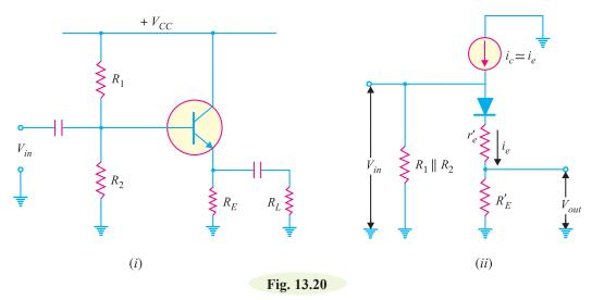
As for CE amplifier, the input impedance of emitter follower is the combined effect of biasing resistors ( $R_1$  and  $R_2$ ) and the input impedance of transistor base [ $Z_{in}$  (*base*)]. Since these resistances
