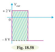
**Note.** It is a biased clamper circuit. It allows a waveform to be shifted above or below (depending upon the polairty of 2 V battery) a dc reference other than 0 V.
