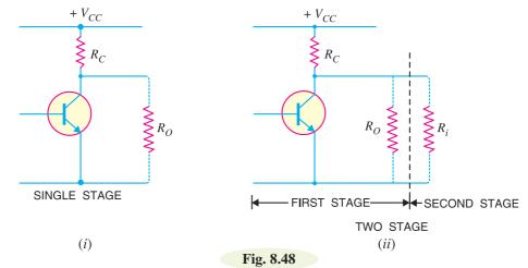
(v) Voltage gain. It is the ratio of change in output voltage  $(\Delta V_{CE})$  to the change in input voltage  $(\Delta V_{BE})$  i.e.
