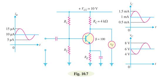
The output voltage,  $v_C = V_{CC} - i_C R_C$
