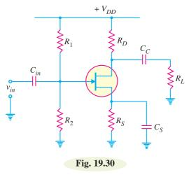
We shall split the JFET amplifier shown in Fig. 19.30 into d.c. and a.c. equivalent circuits. Note that biasing is provided by voltage-divider circuit.
