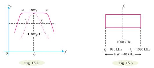
**Illustration**. Consider a tuned amplifier that is designed to amplify only those frequencies that are within  $\pm 20$  kHz of the central frequency of 1000 kHz (*i.e.*,  $f_r = 1000$  kHz). Here [See Fig. 15.3],
