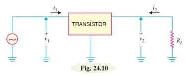
Fig. 24.10 shows the transistor amplifier circuit. There are four quantities required to describe the external behaviour of the transistor amplifier. These are  $v_1$ ,  $i_1$ ,  $v_2$  and  $i_2$  shown on the diagram of Fig. 24.10. These voltages and currents can be related by the following sets of equations :
