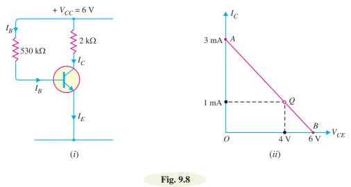
**Operating point Q.** As it is a silicon transistor, therefore,  $V_{BE} = 0.7$ V. Referring to Fig. 9.8 (*i*), it is clear that :
