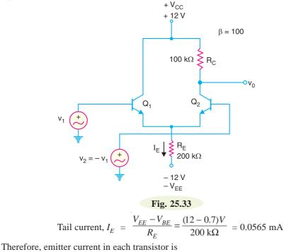
$I_{E1} = I_{E2} = I_E/2 = 0.0565 \text{ mA}/2 = 0.0283 \text{ mA}$
