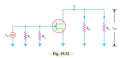
Applying these two steps to the circuit shown in Fig. 19.30, we get the a.c. \*equivalent circuit shown in Fig. 19.32. We can easily calculate the a.c. currents and voltages from this circuit.
