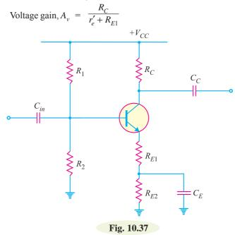
If  $R_{E1} \ge 10 r'_e$ , then the effect of  $r'_e$  is almost negligible and the voltage gain is given by ;
