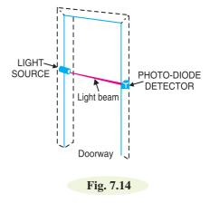
light across a conveyor to a photo-diode. As the object passes, the light beam is broken,  $I_R$  drops to the dark current level and the count is increased by one.
