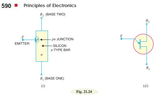
called base leads *base-one*  $B_1$  and *base two*  $B_2$ . Part way along the bar between the two bases, nearer to  $B_2$  than  $B_1$ , a *pn* junction is formed between a *p*-type emitter and the bar. The lead to this junction is called the *emitter lead* E. Fig. 21.24 (*ii*) shows the symbol of unijunction transistor. Note that emitter is shown closer to  $B_2$  than  $B_1$ . The following points are worth noting :
