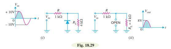
**Solution.** When the diode is connected in parallel with the load, it is called a shunt clipper. During the positive half-cycle of input ac signal, the diode is reverse biased and it will behave as an open. This is shown in Fig. 18.29 (*ii*). With diode as an open,
