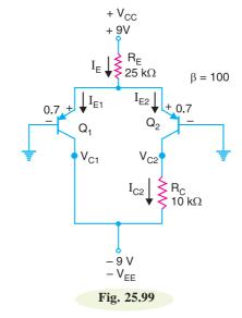
$[V_E = 0.7 \text{ V}; I_E = 0.332 \text{ mA}; I_{E1} = I_{E2} = 0.166 \text{ mA}; I_{C1} = I_{C2} = 0.166 \text{ mA}; I_{B1} = I_{B2} = 1.66 \mu\text{A};$  $V_{C1} = -9 \text{ V}; V_{C2} = -7.34 \text{ V}]$
