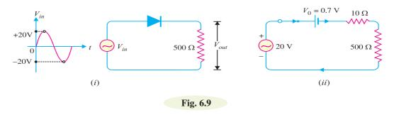
(*i*) The peak current through the diode will occur at the instant when the input voltage reaches positive peak *i.e.*  $V_{in} = V_F = 20$  V.
