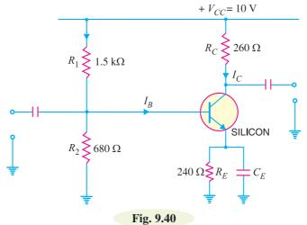
:. Emitter current,  $I_E = \frac{V_2 - V_{BE}}{R_E} = \frac{3.12 - 0.7}{0.24} = 10 \text{ mA}$
