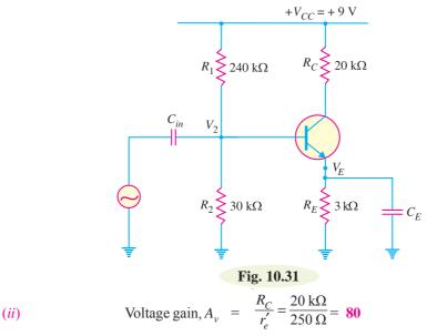
(*iii*) The d.c. voltage across input capacitor is equal to the d.c. voltage at the base of the transistor which is  $V_2 = 1$ V. Therefore, d.c. voltage across  $C_{in}$  is **1V**.
