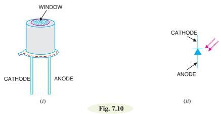
Fig. 7.10 (*ii*) shows the schematic symbol of a photo-diode. The inward arrows represent the incoming light.
