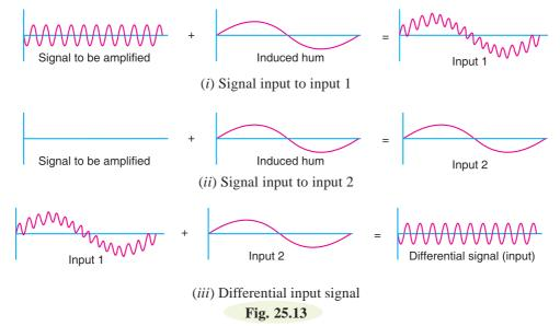
(*i*) In Fig. 25.13(*i*), the signal is applied to input 1 of the *DA*. However, a low frequency *hum* voltage is also induced into the lead wire. This hum is produced due to building and collapsing magnetic field generated by adjacent conductor carrying 50Hz current. The resultant waveform is shown in Fig. 25.13 (*i*). If this waveform is amplified by a conventional amplifier, the 50 Hz hum in the output will be stronger than the desired signal.
