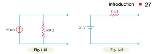
Convert the voltage source in Fig. 1.49 into equivalent current source. [3 mA in parallel with 8 kΩ]
