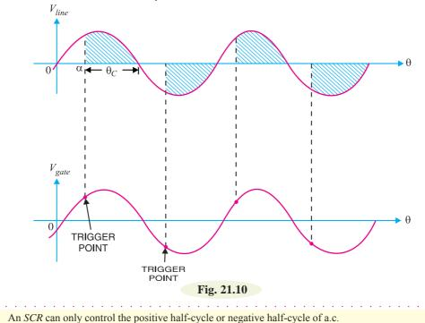
\*\* An *SCR* is a controlled unidirectional switch because it can conduct only in one direction.
