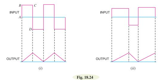
(*ii*) When input is rectangular wave. When the input fed to an integrating circuit is a rectangular wave, the output will be a triangular wave as shown in Fig. 18.24 (*ii*).
