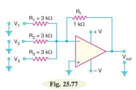
(*ii*) The ratio of any input resistor to the feedback resistor is equal to the number of input circuits.
