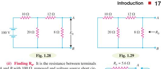
A and B with 100  $\Omega$  removed and voltage source short circuited as shown in Fig. 1.29.
