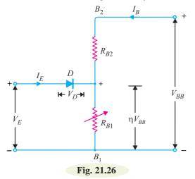
(a)  $R_{B2}$  is the resistance of silicon bar between  $B_2$  and the point at which the emitter junction lies.
