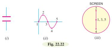
The result is that the spot moves up and down at the same rate as the frequency of the applied voltage. As the frequency of applied voltage is 50 Hz, therefore, due to persistence of vision, we will see a continuous vertical line 2 - 1 - 4 on the screen as shown in Fig. 22.22 (*iii*). The line gives no indication of the manner in which the voltage is alternating since it does not reveal the waveform.
