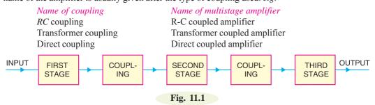
(*i*) In *RC* coupling, a capacitor is used as the coupling device. The capacitor connects the output of one stage to the input of the next stage in order to pass the a.c. signal on while blocking the d.c. bias voltages.
