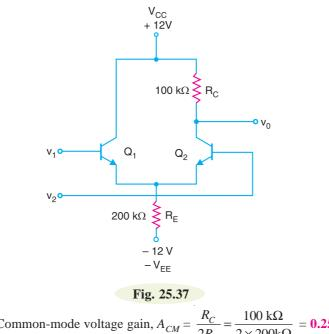
**Solution.** (*i*) Common-mode voltage gain,  $A_{CM} = \frac{R_C}{2R_E} = \frac{100 \text{ k}\Omega}{2 \times 200 \text{k}\Omega} = 0.25$
