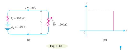
(*i*) Due to high internal resistance of the source, the load current remains essentially constant as the load  $R_L$  is varied.
