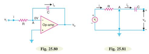
**Circuit Analysis.** Since point *A* in Fig. 25.80 is at virtual ground, the \*virtual-ground equivalent circuit of operational integrator will be as shown in Fig. 25.81. Because of virtual ground and infinite impedance of the *OP*-amp, all of the input current *i* flows through the capacitor *i.e.*  $i = i_c$ .
