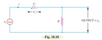
Fig. 18.18 shows a typical differentiating circuit. The output across R will be the derivative of the input. It is important to note that merely using voltage across R does not make the circuit a differentiator; it is also necessary to set the proper circuit values. In order to achieve good differentiation, the following two conditions should be satisfied :
