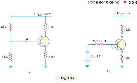
$$R_0 = \frac{R_1 R_2}{R_1 + R_2} = \frac{10 \times 5}{10 + 5} = \frac{50}{15} = 3.3 \text{ k}\Omega$$
