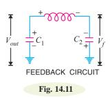
duced by  $C_1 - C_2$  voltage divider. In this way, feedback is properly phased to produce continuous undamped oscillation.
