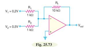
**Solution.**  $R_f = 10 \text{ k}\Omega$  and  $R_1 = R_2 = R = 1 \text{ k}\Omega$ . Therefore, gain of the amplifier  $= -R_f/R = -10 \text{ k}\Omega/1\text{k}\Omega = -10$ .
