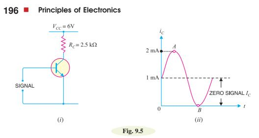
Thus, the maximum collector current allowed during any part of the signal is 2 mA. If the collector current is allowed to rise above this value,  $V_{CE}$  will fall below 1 V. Consequently, value of  $\beta$  will fall, resulting in unfaithful amplification.
