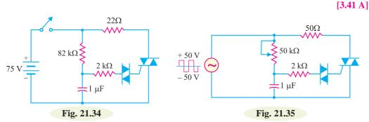
7. If the triac of Fig. 21.35 has1V across it when it is conducting, what is the maximum current through the 50Ω?
