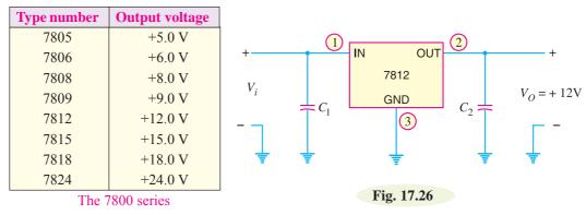
Fig. 17.26 shows how the 7812 *IC* is connected to provide a fixed d.c. output of + 12V. The unregulated input voltage  $V_i$  is connected to the *IC's IN* terminal and the *IC's OUT* terminal provides + 12V. Capacitors, although not always necessary, are sometimes used on the input and output as shown in Fig. 17.26. The output capacitor ( $C_2$ ) acts basically as a line filter to improve transient response. The input capacitor ( $C_1$ ) is used to prevent unwanted oscillations.
