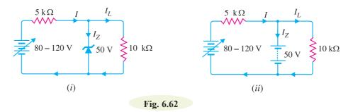
**Maximum zener current.** The zener will conduct \*maximum current when the input voltage is maximum *i.e.* 120 V. Under such conditions :
