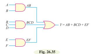
The variables A and B are ANDed to produce AB, B, C and D are ANDed to produce BCD and E and F are ANDed to produce EF. The input to OR gate is AB, BCD and EF so the output of this gate is the ORing of the inputs *i.e.*
