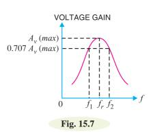
The practical importance of bandwidth of tuned amplifiers is found in communication system. In radio and TV transmission, a very high frequency wave, called *carrier wave* is used to carry the audio or picture signal. In radio transmission, the audio signal has a frequency range of 10 kHz. If
