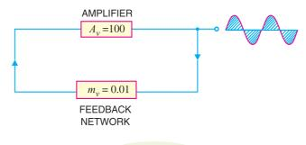
undamped oscillations,  $m_v A_v = 1$  or  $m_v \times 100 = 1$  or  $m_v = 0.01$ . This is illustrated in Fig. 14.8. Since the condition  $m_v A_v = 1$  is met in the circuit shown in Fig. 14.8, it will produce sustained oscillations.
