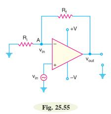
**Voltage gain.** If we assume that we are not at saturation, the potential at point A is the same as  $V_{in}$ . Since the input impedance of *OP*-amp is very high, all of the current that flows through  $R_f$  also flows through  $R_i$ . Keeping these things in mind, we have,
