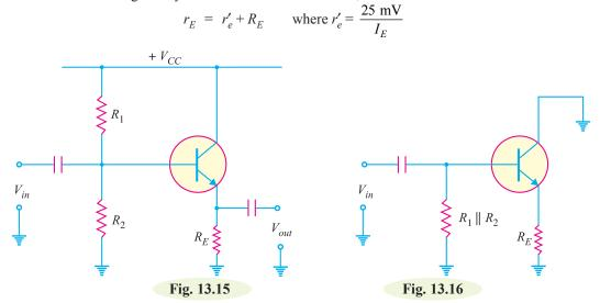
In order to find the voltage gain of the emitter follower, let us replace the transistor in Fig. 13.16 by its equivalent circuit. The circuit then becomes as shown in Fig. 13.17.
