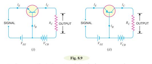
1. Current amplification factor ( $\alpha$ ). It is the ratio of output current to input current. In a common base connection, the input current is the emitter current  $I_E$  and output current is the collector current  $I_C$ .
