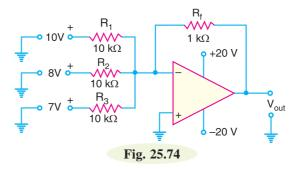
**Solution.**  $R_f = 1 \text{ k}\Omega$  and  $R_1 = R_2 = R_3 = R = 10 \text{ k}\Omega$ . Therefore, gain of the amplifier  $= -R_f/R = -1 \text{ k}\Omega/10 \text{ k}\Omega = -1/10$ .
