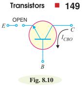
age of it, as a result of electron-hole combinations occurring in base area, gives rise to base current. Moreover, as the collector-base junction is reverse biased, therefore, some leakage current flows due to minority carriers. It follows, therefore, that total collector current consists of :
