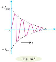
**Frequency of oscillations.** The frequency of oscillations in the tank circuit is determined by the constants of the circuit viz L and C. The actual frequency of oscillations is
