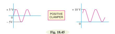
A clamping circuit (or a clamper) essentially adds a *d.c.* component to the signal. Fig. 18.45 shows the key idea behind clamping. The input signal is a sine wave having a peak-to-peak value of 10 V. The clamper adds the *d.c.* component and pushes the signal upwards so that the negative peaks fall on the zero level. As you can see, the waveform now has peak values of +10 V and 0 V.
