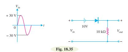
**Solution.** For any value of  $V_{in} > 10V$ , the ideal diode is forward biased and  $V_{out} = V_{in} - 10$ . For example, at  $V_{in} = 15V$  [See Fig. 18.36 (i)],  $V_{out} = 15 - 10 = 5V$ .
