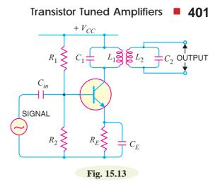
load resistance is coupled into the primary tank circuit  $L_1C_1$  and affects the primary circuit in exactly the same manner as though a resistor had been added in series with the primary coil  $L_1$ .
