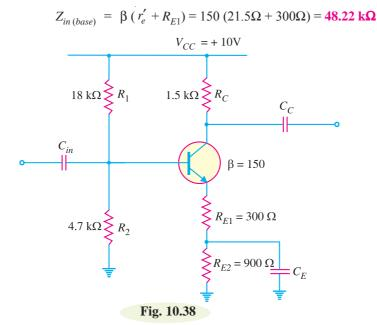
**Example 10.22.** Determine the change in voltage gain for the amplifier in example 10.21 when  $r'_e$  doubles in value.
