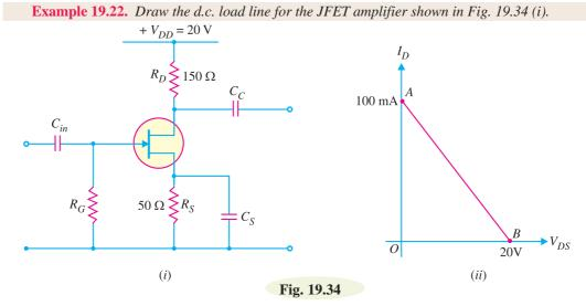
**Solution.** To draw d.c. load line, we require two end points *viz.*, max  $V_{DS}$  and max.  $I_D$  points. Max.  $V_{DS} = V_{DD} = 20$ V
