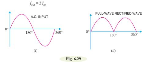
For example, if the input frequency to a full-wave rectifier is 100 Hz, then the output frequency will be 200 Hz.
