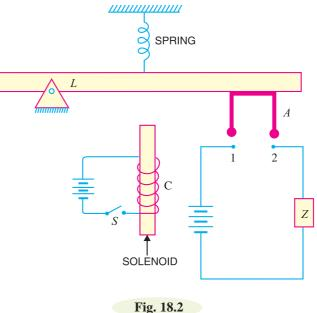
lenoid is de-energised and the spring pulls the lever and hence the armature A upwards. Consequently, the relay contacts 1 and 2 are opened and current flow in the circuit is interrupted. In this way, a relay acts as a switch.
