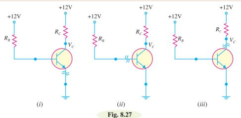
**Solution.** \*Fig 8.27 shows the open circuit failures in a transistor. We shall discuss the circuit behaviour in each case.
