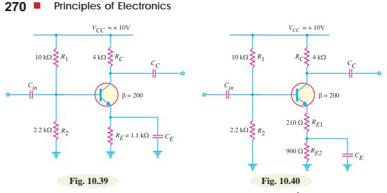
**Solution.** Both the circuits have the same value of a.c. emitter resistance  $r'_e$ . Therefore, following the standard procedure for finding  $r'_e$  gives us a value of \*25 $\Omega$  for both circuits.
