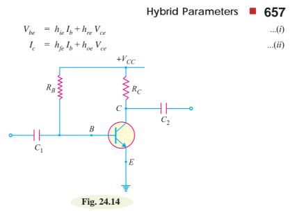
(i) Determination of  $h_{fe}$  and  $h_{ie}$ . In order to determine these parameters, the output is a.c. short circuited as shown in Fig. 24.15 (i). This is accomplished by making the capacitance of  $C_2$ deliberately large. The result is that changing component of collector current flows through  $C_2$  instead of  $R_c$  and a.c. voltage developed across  $C_2$  is zero *i.e.*  $*V_{ce} = 0$ .
