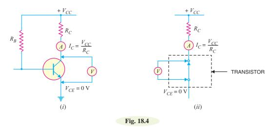
(*ii*) When the input base voltage is positive enough that transistor saturates, then  $I_{C(sat)}$  will flow through  $R_C$ . Under such conditions, the entire  $V_{CC}$  will drop across collector load  $R_C$  and output the collector current will not be zero since a little leakage current always flows even when the base input voltage is negative or zero.
