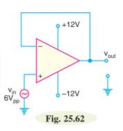
(ii) Since  $A_{CL} = 1$  for the circuit,  $v_{out} = v_{in}$ . Therefore, peak output voltage  $(V_{pk})$  is one-half of  $6V_{pp}$  *i.e.*,  $V_{pk} = 6/2 = 3$  V. The maximum operating frequency  $(f_{max})$  is given by ;
