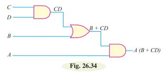
The variable *C* is ANDed with *D* and its output is *CD*. Then *CD* is ORed with *B*, giving an output (B + CD). This sum is then ANDed with *A*, resulting in the following Boolean expression :
