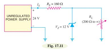
The maximum load current occurs when  $R_L = 200 \Omega$ .
