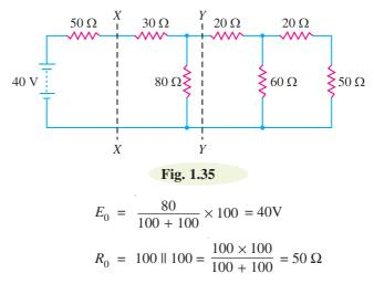
**Solution.** We shall simplify the circuit shown in Fig. 1.34 by the repeated use of Thevenin's theorem. We first find Thevenin's equivalent circuit to the left of \*XX.
