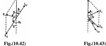
Since  $R_a$  is very small as compared to  $X_s$ ,  $\theta$  is nearly 90° so that the current  $I_{sy}$  is almost in phase with  $E_1$  and in phase opposition to  $E_2$ . This means that machine 1 is generating and machine 2 is motoring. Consequently, machine 1 tends to slow down and machine 2, by accepting power, tends to accelerate. This restores the status quo i.e., synchronism is re-established.
