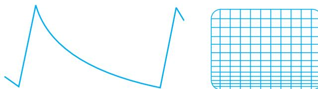
Fig. 19.3 (b). Non-linear sawtooth causing crowding of lines at the bottom of the raster.
