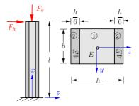
Determine the normal stress distribution in the cross section at the clamping.
