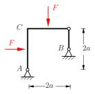
**Solution** We use the principle of virtual forces, neglecting shear, tension and torsion contributions:
