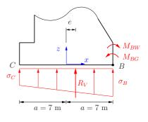
$$\underline{\sigma} = \frac{-3990}{14} + \frac{-1685}{228.67} x = \underline{-285 - 7.37 x \text{ kN/m}^2}.$$
