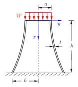
**Solution** As the weight W is the only acting external load, the normal force N is constant (compression):
