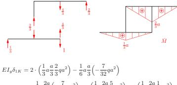
$$\begin{aligned} &+\frac{1}{6}a\frac{2a}{3}\left(-\frac{7}{32}qa^2\right) + 2\left(\frac{1}{3}a\frac{2a}{3}\frac{5}{6}qa^2\right) + 2\left(\frac{1}{3}a\frac{2a}{3}\frac{1}{8}qa^2\right) \\ &= qa^4\left(\frac{4}{27} - \frac{7}{576} - \frac{14}{576} + \frac{10}{27} + \frac{1}{18}\right) \\ &= \frac{929}{1728}qa^4. \end{aligned}$$
