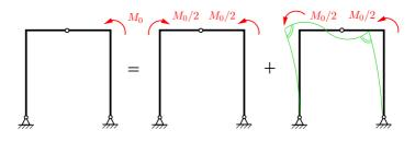
The antisymmetric loading causes no reciprocative rotation at the hinge. For the symmetric loadign it suffices to consider half of the frame structure. The rotation  $\psi$  results solely from the bending of the vertical post (only a normal force occurs in the horizontal beam). Thus from the table on page 62 (load case no. 4 with  $\beta = 1$  and  $\alpha = 0$ ) we obtain
