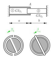
**Solution** In the assembled state both shafts are loaded by the torque  $M_T$ . We cut the system at position A and determine the angle of twist of ① and ② separately:
