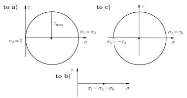
Note: In case **b**) Mohr's circle degenerates to a single point along the  $\sigma$ -axis!
