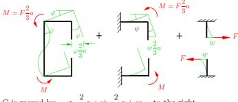
C is moved by  $\varphi \cdot \frac{2}{3}a + \psi \cdot \frac{2}{3}a + w$  to the right, D is moved by  $\varphi \cdot \frac{2}{3}a + \psi \cdot \frac{2}{3}a + w$  to the left.
