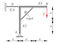
**Solution** The system is statically determinate supported, but due to the rigid truss internally statically indeterminate. To compute the force  $S_2$  in bar <sup>(2)</sup> we use the following "0"- and "1"-systems. The reaction forces and the force in bar <sup>(1)</sup> can be determined from equilibrium conditions.
