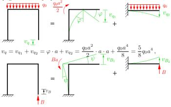
$$v_B = v_{B_1} + v_{B_2} = \psi \cdot a + v_{B_2} = Ba \cdot a \cdot a + B \frac{a^3}{3} = \frac{4}{3} Ba^3.$$
