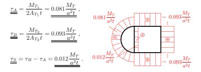
Equalizing the maximum shear stress with the admissible shear stress
