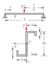
**Solution** The displacement can be determined with regards to the y, z-axes, or with regard to the principal axes. We want to consider both possibilities.
