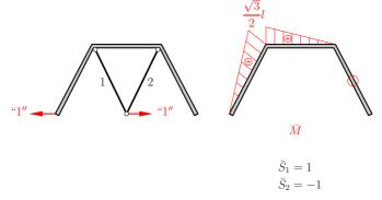
Using the "0"- and "1"-system we determine the horizontal displacement
