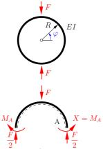
the fact that the slope at A has to vanish (symmetry!). Use of the principle of virtual forces yields:
