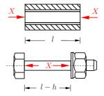
The length changes have to be adjusted in such a way that casing and screw have the same length. Therefore compatibility can be written as
