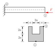
**Solution** As the neutral axis is passing trough the centroids of the cross sections, we first determine the position of the centroid:
