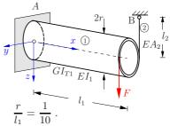
**Solution** The system is statically indeterminate. We choose the reaction force in B as statically redundant force. This leads to the following "0"- and "1"-system:
