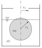
**Solution** The ball has to submerge to a depth that just closes the opening when the container is full. The buoyancy force is than  $\rho_F g V_1$ , where  $V_1$  is the volume of the displaced fluid (spherical segment). The buoyancy force has to be equal to the weight of the ball
