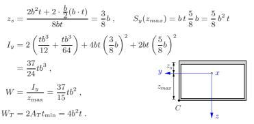
Using bending moment, torque, shear force in the clamped support
