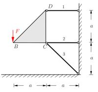
**Solution to a)** The system is statically determinately supported. The forces in the bars follow immediately from the equilibrium conditions:
