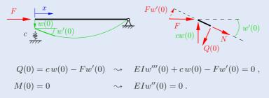
Four characteristic boundary conditions establish the  ${\bf Euler \ buckling \ cases:}$
