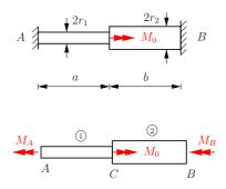
**Problem 4.10** A shaft is clamped at both ends and loaded along part b of its length l by a constant distributed torque  $m_0$ .
