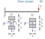
**Solution** With V = F the shear stress in the bonding layer becomes in general  $(z = z_l)$
