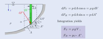
The resulting horizontal component of the fluid pressure  $F_H$  is equal to the product of the vertically projected area  $A^*$  and the pressure  $p_{C^*}$  in the centroid of the projected area.
