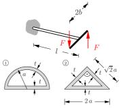
**Solution** The torque  $M_T = 2bF$  is constant along the length of the shaft. Stress and twist are determined from
