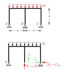
Using the principle of virtual forces we construct the following basic and auxiliary systems :
