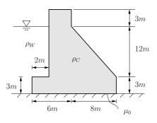
Given:  $\rho_C = 2.5 \cdot 10^3 \text{ kg/m}^3$ ,  $\rho_W = 10^3 \text{ kg/m}^3$ ,  $\mu_0 = 0.5$ ,  $g = 10 \text{ m/s}^2$
