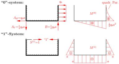
From the condition, that difference in the displacement of the frame and the end of the truss has to vanish,
