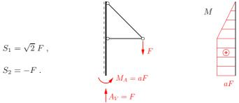
The vertical displacement can be calculated by loading the system with a force "1" in vertical direction. By replacing F by "1" the above results can be used:
