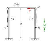
b) The force F is removed after assembly. Determine the force in the rope and the moments at both supports.
