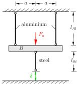
Given:  $l_{Al} = 1 \text{ m}, d_{Al} = 2 \text{ mm}, E_{Al} = 0.7 \cdot 10^5 \text{ MPa}, l_{St} = 1.5 \text{ m}, d_{St} = 2 \text{ mm}, E_{St} = 2.1 \cdot 10^5 \text{ MPa}, \delta = 5 \text{ mm}$ .
