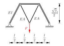
**Solution** Since the vertical displacement  $v_F$  of the load has the same direction as load F, we can determine  $v_F$  by the conservation of energy:
