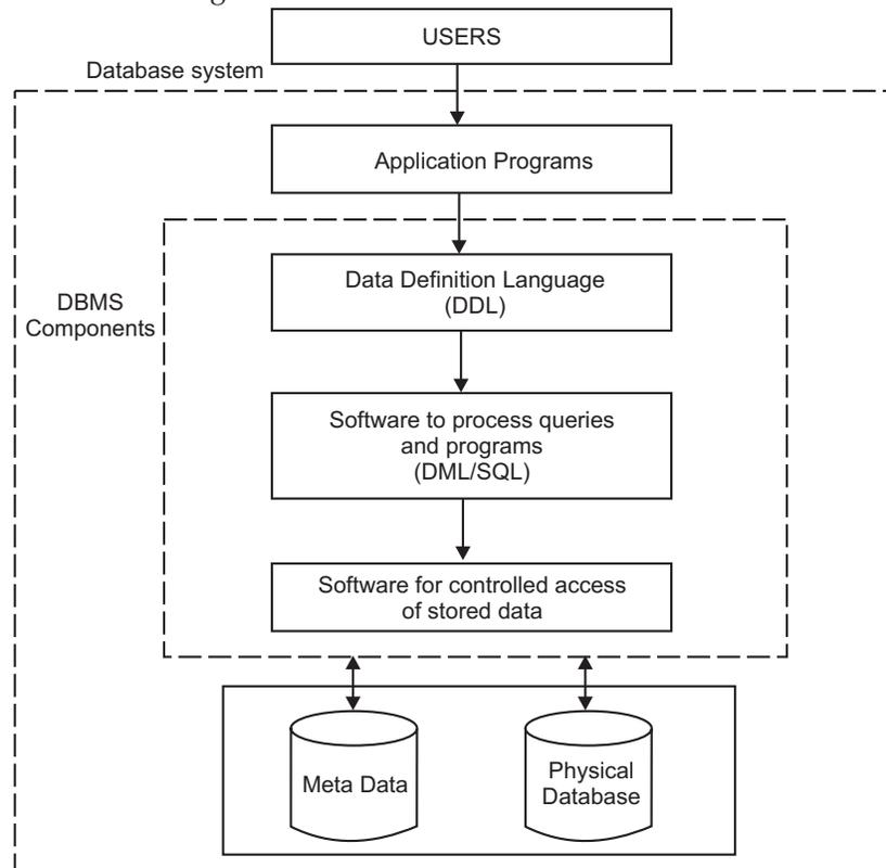
FIGURE 1.2. Components of DBMS.
