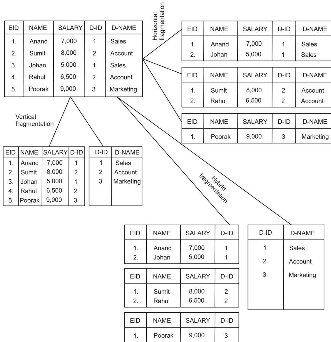
FIGURE 12.5. Demonstration of horizontal, vertical and hybrid fragmentation.
