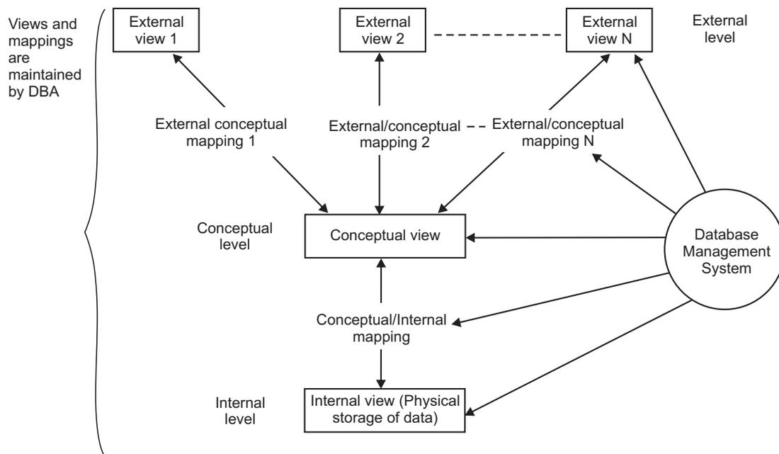
FIGURE 1.7. Three level architecture of DBMS.
