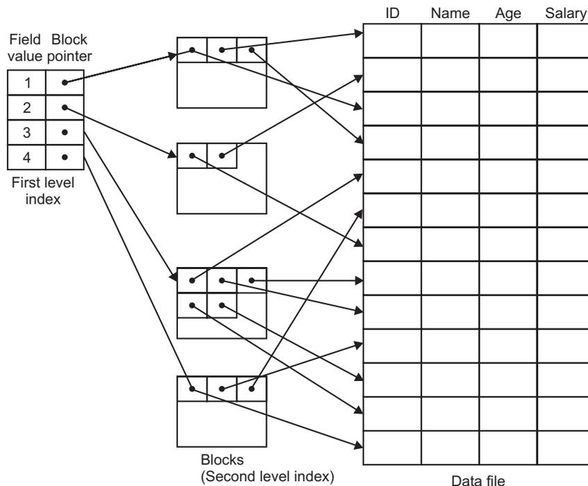
FIGURE 3.22. Multilevel indexing.
