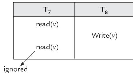
**FIGURE 8.15.** Schedule for transactions  $T_7$  and  $T_8$ .
