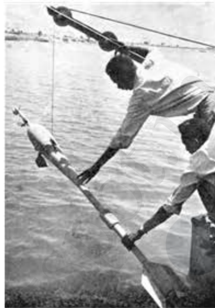
Fig. 4.10 Propeller-type Current Meter—Neyrtec Type with Sounding Weight
