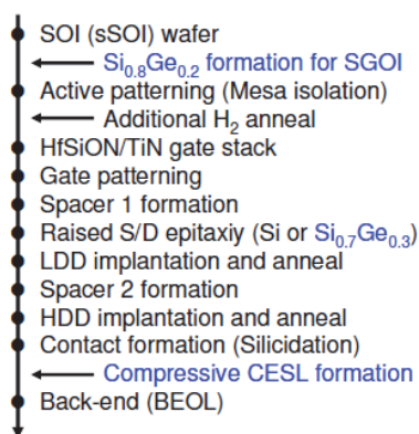
Figure 9.37. Process integration schematic of MOSFETs. After M. Koyama, Electrical characterization of interface properties in nano-scaled MOSFET devices based on low-frequency fluctuations, PhD Thesis, Universite Grenoble Alpes, 2015.
