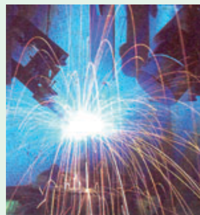
An electric arc is produced when electricity is passed between two electrodes
